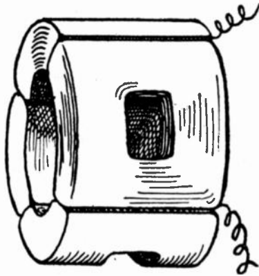
FIG. 4. DETAIL OF SCANNING COIL
