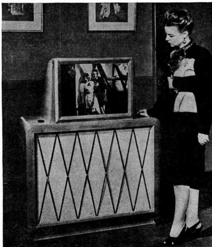
FIG. 5.—RCA improved home television receiver. Shown here is an improved engineering development model home television receiver built by the RCA Victor Division of the Radio Corporation of America. It provides large-screen television for the home, with bright, clear, high-definition pictures about the size of a standard newspaper. This type of home television receiver projects moving images on a built-in screen by means of a unique projection system employing a spherical mirror and a molded plastic aspherical lens. The system was developed by RCA before the Second World War. Also incorporated in the new receiver is an automatic control system which virtually eliminates picture distortion caused by noise interference. (RCA Victor Division, Radio Corporation of America, Camden, N. J.)
