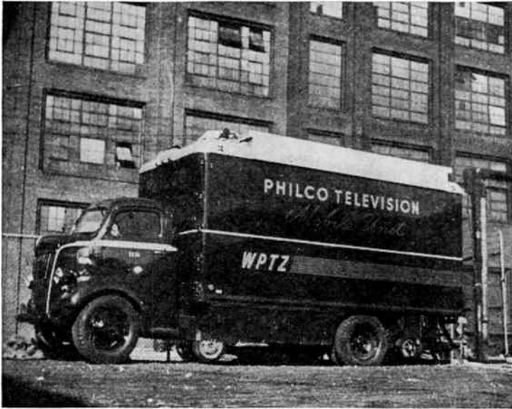
FIG. 101.—Mobile unit of Philco television station WPTZ, Philadelphia, ready at all times to transport the remote pickup television cameras and equipment to the scene to be televised. ( Philco Corporation. )
