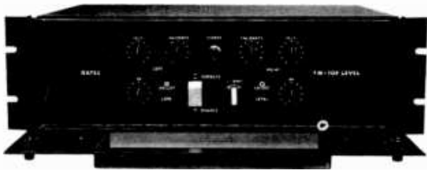
Fig. 10-16. A dual-channel FM program level control unit for stereo and monaural service.
