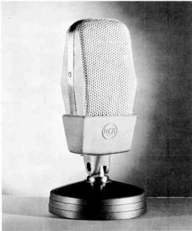
Fig. 12-7. A typical velocity microphone.
