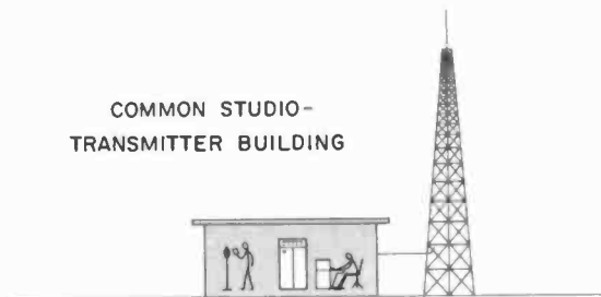
Fig. 1-3. In many stations, studio and transmitter facilities are combined within a common building.
