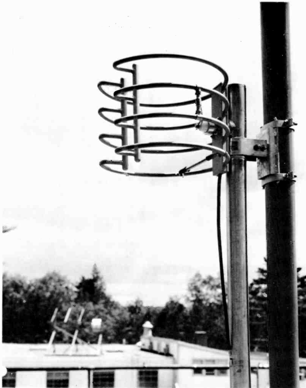
Fig. 8-3. Radiating element of a ring-type horizontally-polarized FM antenna.
