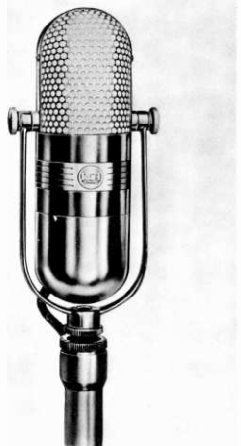
Fig. 12-2. A polydirectional microphone.
