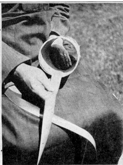
As each cut is made, it is "backed" up with gummed paper so that the form can be taken apart without wrecking the finished inductance
