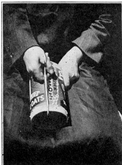
The winding form is slit in three sections with a scissors, cutting the cardboard lengthwise. A common Quaker Oats box serves the purpose
