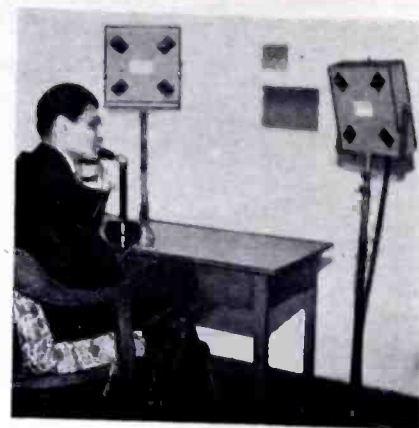
Seated at the table and carrying out a visio-telephony conversation. Note the banks of photo-electric cells and the aperture cut in the wall.
