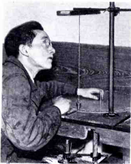
The author illustrating the method of using the plumb bob for adjusting the lens scanning disc.
