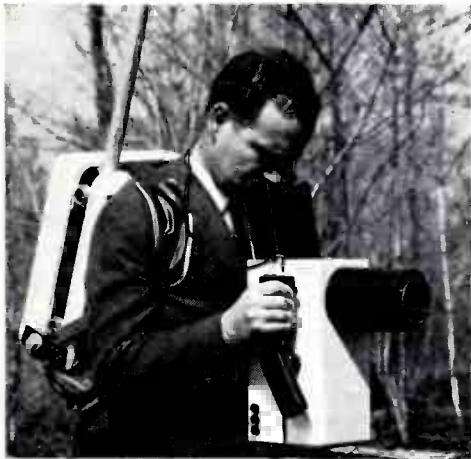
Cameras for special television needs. The sophisticated Minicam III multi-purpose wireless camera may be used at waist-level, eye-level, or periscope viewing positions.
