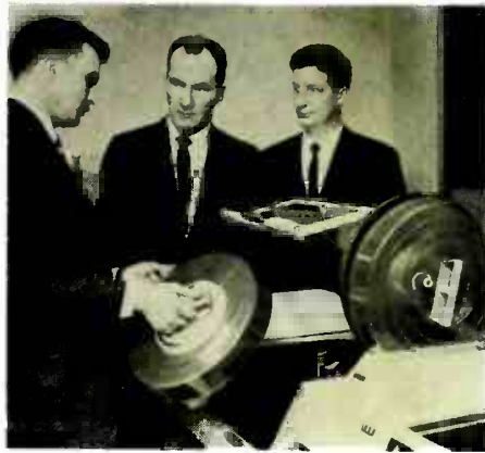
Vast quantities of data are stored. Each of five disk storage drives, such as Roberts displays here, stores seven million characters, instantaneously available to a pick-up arm that reads and writes at the rate of 156,000 characters a minute.
