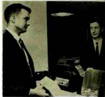
The cards are fed into a reader by computer operator Clyde Roberts (l) as Bowlin looks on. The machine reads at the rate of 600 cards a minute.
