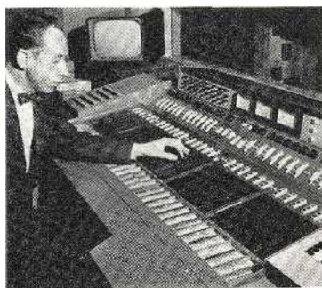
McCurdy SS4724 solid-state custom audio console is part of Canadian equipment line marketed through Visual Electronics Corp.
