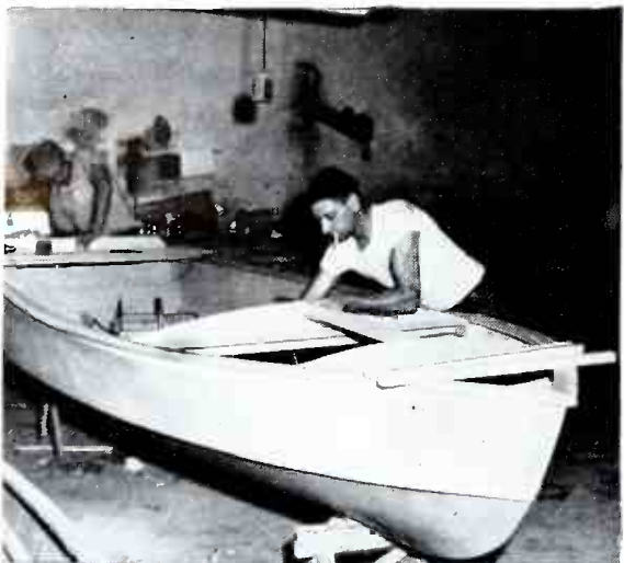
DOLPHIN CRAFT are reinforced fiberglass plastic boats, moulded in one piece, trimmed with mahogany, oak or cypress, made in Jacksonville at the rate of 50 a week.
