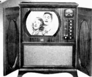
THE SENSITUNER, above—just one example of the extra television values that make the DuMont franchise so satisfying. An improvement on the famous DuMont Imputuner,\* the Sensituner has added a fourth tuned circuit which gives greatly increased gain and selectivity. This extra circuit uses every bit of the signal and greatly improves the signal-to-noise ratio—an important feature particularly valuable in weak signal areas.
