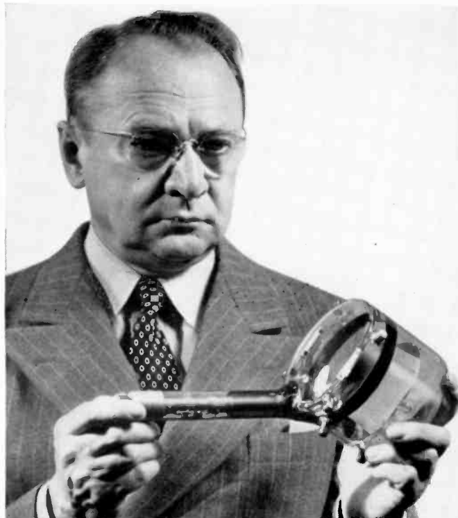
Dr. V. K. Zworykin of RCA Laboratories with his iconoscope tube. Its successor, the image orthicon, has been developed by RCA scientists to have up to 1000 times greater sensitivity.
