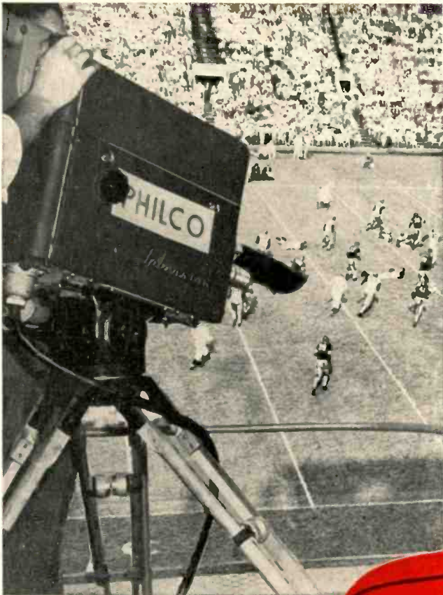
RCA image-orthicon cameras, standard equipment for the new truck, rival the human eye in sensitivity—eliminate fading of sports events. Shown above as used by Philco's WFIZ to pick up a Penn game at Franklin Field, Phila.
