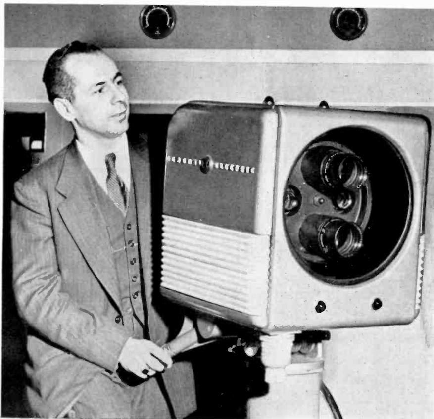
General Electric's new lightweight television camera has two sets of turret-mounted lenses, and is equipped with finger-tip controls. A silent electric hydraulic system, foot-operated, gives flexibility of elevation controls. Lenses are focused by twisting the rotating grip on the right handle, as illustrated.
