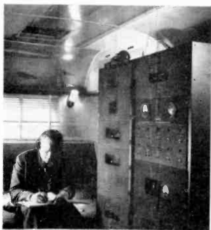
Inside of trailer. At left operator checking on telephone how transmitter signal is being received at next station. At right receiving and outgoing picture monitors.
