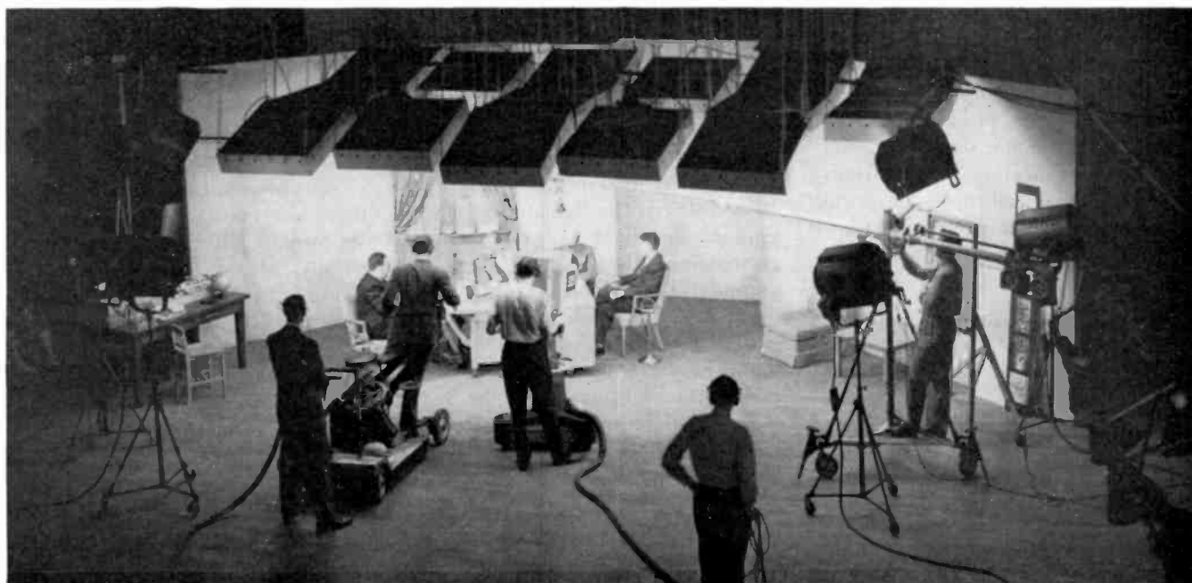
Illustrated at top of picture are box-like holders with fluorescent lights. The large floor units on sides are the arc lamps. These two forms of lighting are most used at CBS, although birdeyes are used occasionally.
