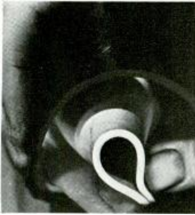
Comparison of Silastic (white), which can remain soft and flexible after 90 days at 300° F. and synthetic organic rubber which has become brittle after one day at 300° F.
