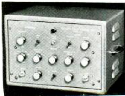
Berkeley Scientific double-pulse generator
