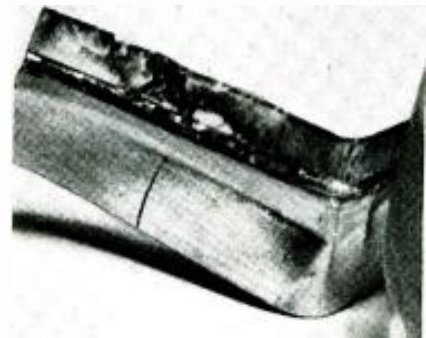
Figure 10 A 2 1/2" diameter ceramic cylinder with brazed-on metal headers.
