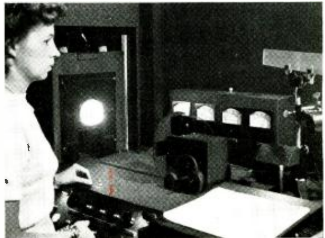
Checking color content and screen coating of picture tubes to assure good black-and-white reproduction. Operator notes the ratio of green, blue and amber against a standard illuminant. (Courtesy Philco)
