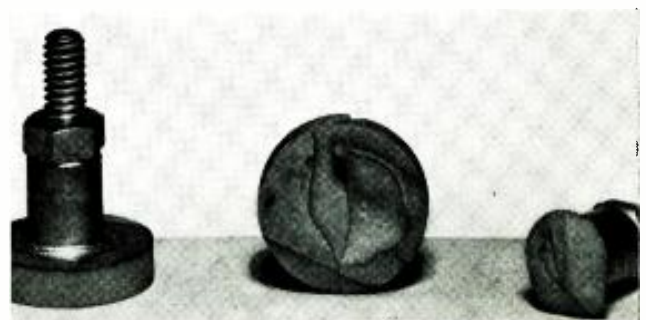
Figure 6 Metal-ceramic butt brazed seal, before and after a tensile test.
