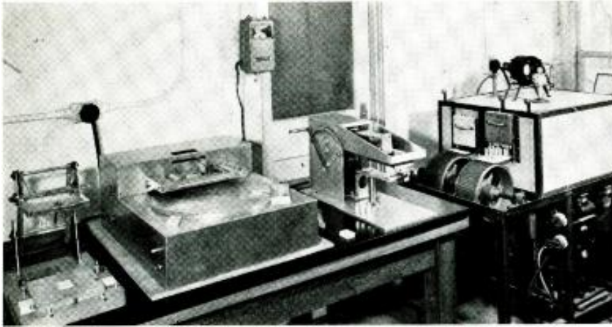
Special equipment for printed-circuit fabrication, designed and constructed at the National Bureau of Standards. Equipment at left are flat-bed metallizing presses of hand operated and motor driven automatic type. A metallizing press for cylindrical work is the third item on the table and at extreme right is a continuous furnace.
