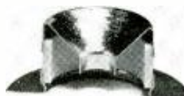
Metallized ceramic cylinder before brazing.
