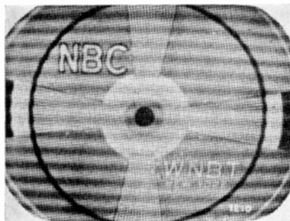
Figure 5 Sound bar pattern in picture caused by tone from the transmitter entering the picture circuit.
