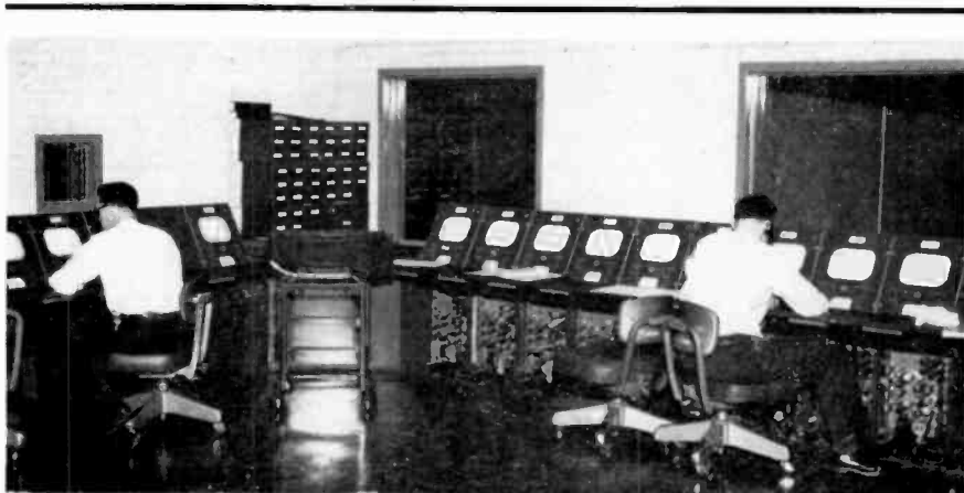
STUDIO AND FILM CAMERA SHADING CONTROLS are located away from the director's booth, camera shading equipment operators are in contact with the director by intercom.
