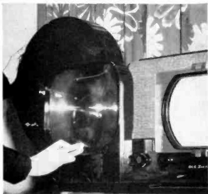
CONVERTER FOR CBS SYSTEM is a synchronized color-filter wheel placed in front of picture tube. Cost to convert present sets would be only ten to fifty dollars it is claimed.
