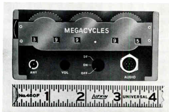
Artist's rendering of the top of the AN/PRC-66 transceiver shows freq. selectors for 3500 UHF channels and other controls.
