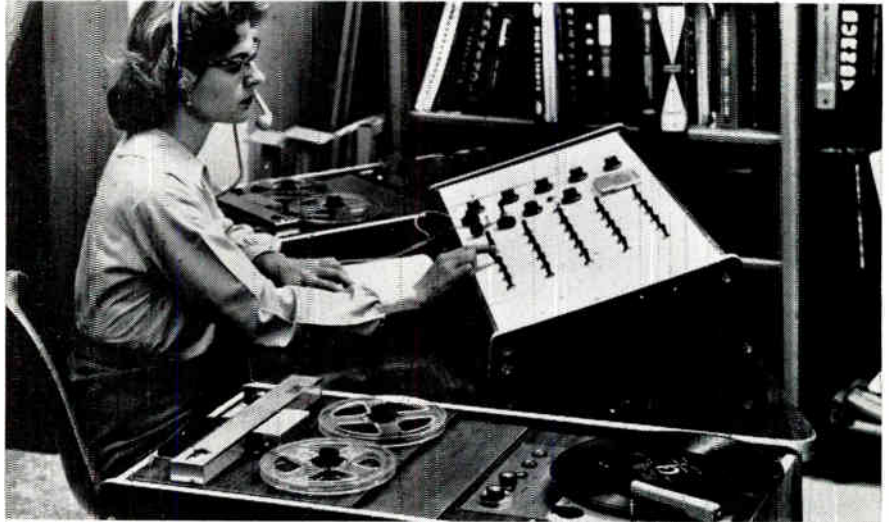
Customized console for new RL-6800 Learning Center developed by Educational Electronics Div., Dage-Bell Corp. In this modular add-on audio system student recorders and amplifiers are in remote compact cabinet under teacher control. Cabinet may house as many as 18 recorders. All student tape deck functions are under the instructor's control.
