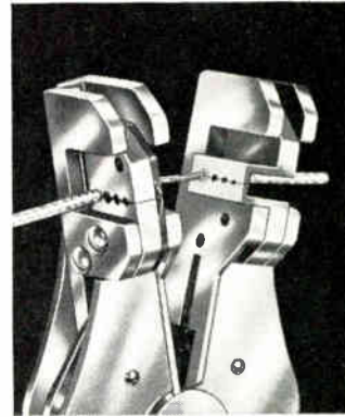
4. End of squeeze. As jaws open, moving gripper removes slug. Stationary collet-blade retains stripped lead. No blade scrapes along conductor.
