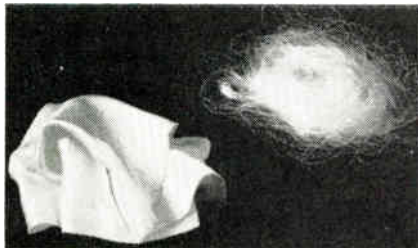
FIBER for ablative and radome applications. Comes in yarn, roving, wool and matt, readily fabricated into cloth or tape.
