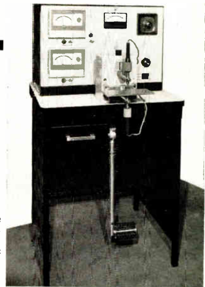
This tape cable welder was developed by ELCO, with the assistance of WEMS.
