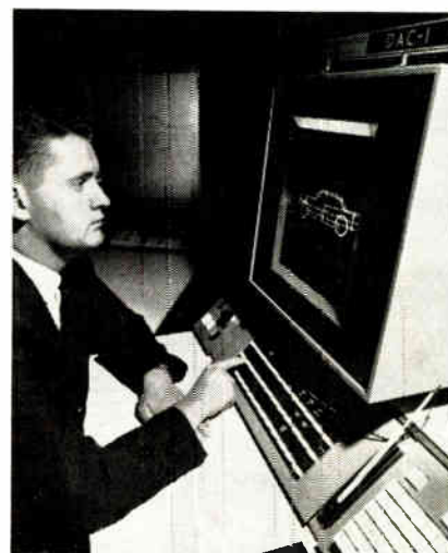
Computer programmer at General Motors Research Laboratories takes role of automotive designer to test out new GM DAC-1 system. The large and complex computer system features a graphic console and image processor. Console monitors and controls computer progress on a design problem. At any design stage, designer may request a permanent photo copy of a new drawing using the image processor.
