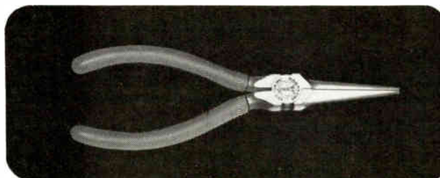
D310-6C Slim Long Nose Plier. Handles are yellow plastisol covered. Supplied with coil spring to keep jaws open.
