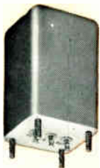
560 — Telemetering low pass filter. Available from 400 to 70 KC. \pm 7.5\% bandwidth flat to 1 db. Attenuation greater than 35 db beyond the 2nd harmonic of \pm 7.5\% frequency. Impedance 47K ohms. MIL-F-18327B. Wt. 0.8 oz.
