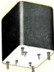
Low frequency band pass filter. Designed for 2.5 cps center frequency. At 2 to 3 cps within 3 db. At 1.5 cps and lower, and 4 cps and higher, greater than 30 db. Source and Load 10K ohms. Size: 4 x 4-11/16 x 6". MA MIL case, MIL-F-18327B.
