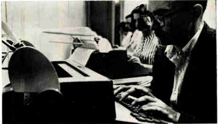
Employees at IBM's Thomas J. Watson Research Center shown taking experimental courses via computer assisted instruction. A teacher's instruction, questions and guidance can be stored and presented to student through typewriter consoles. Replies are put on typewriter and analyzed by computer. Course material can be tailored to needs.
