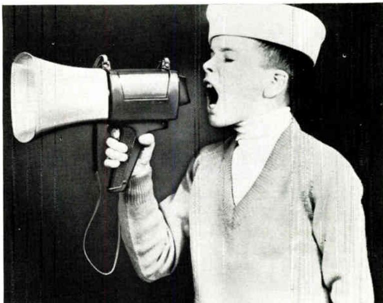
Portable, transistorized megaphone transmits audio, blinker and Morse code. Average range is 100 yards. Has selector switch and volume control.
