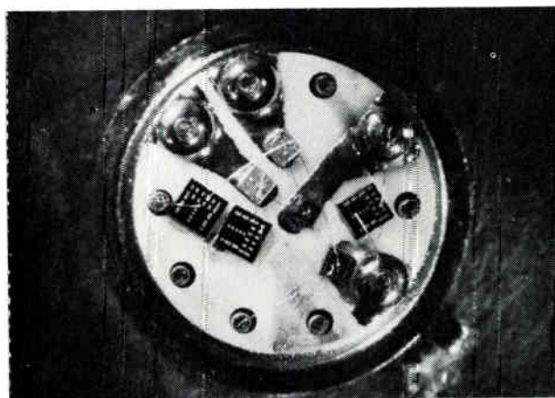
Fig. 4—Hybrid (multichip) technique uses component chips, diffused or thin-film, fastened to ceramic substrate, and interconnected by combination of metallized patterns and wire bonds.
