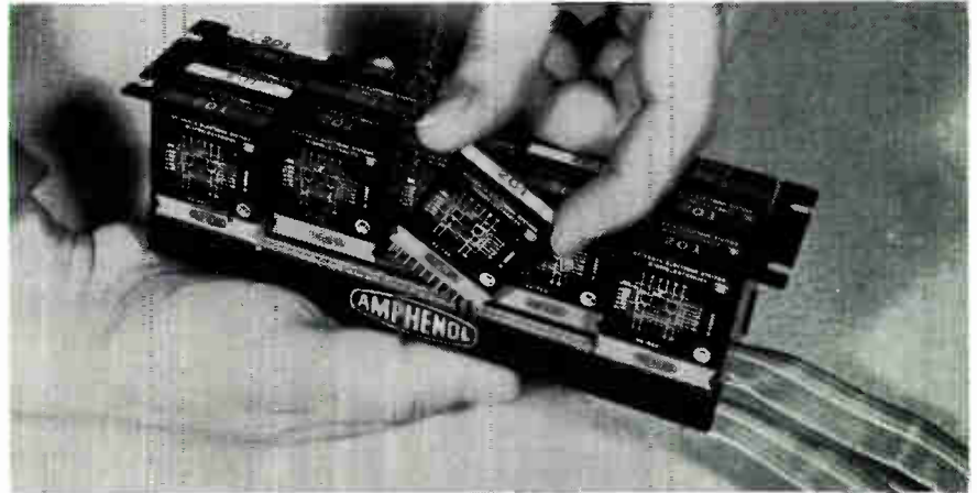
Fig. 5: In this module-to-motherboard configuration, interconnections may be soldered, welded, or crimped. Wire wrapping and mating connectors may also be used.
