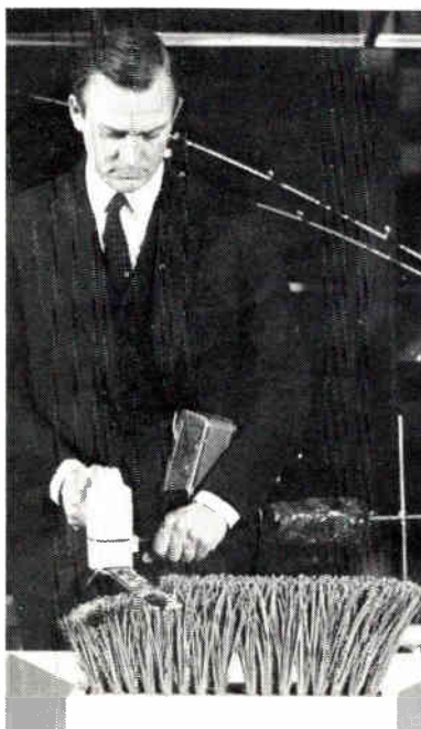
A variety of power tools have been made portable by battery power packs such as the one seen here.
