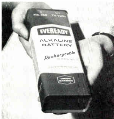
This rechargeable alkaline battery is used to power miniature TV sets.
