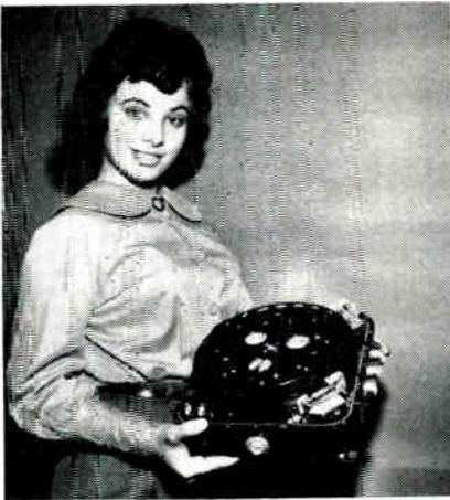
Miss B. Miller holds tape recorder built by RCA Surface Communications Div. for Gemini spacecraft. The 10 w. recorder will tape 4 hrs. of telemetry data aboard craft, play it back in 11 min. The unit weighs 12 lbs.
