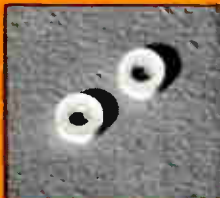
Thickness .089 \pm .001 Hole .125 \begin{matrix} +.0015 \\ -.0000 \end{matrix}
