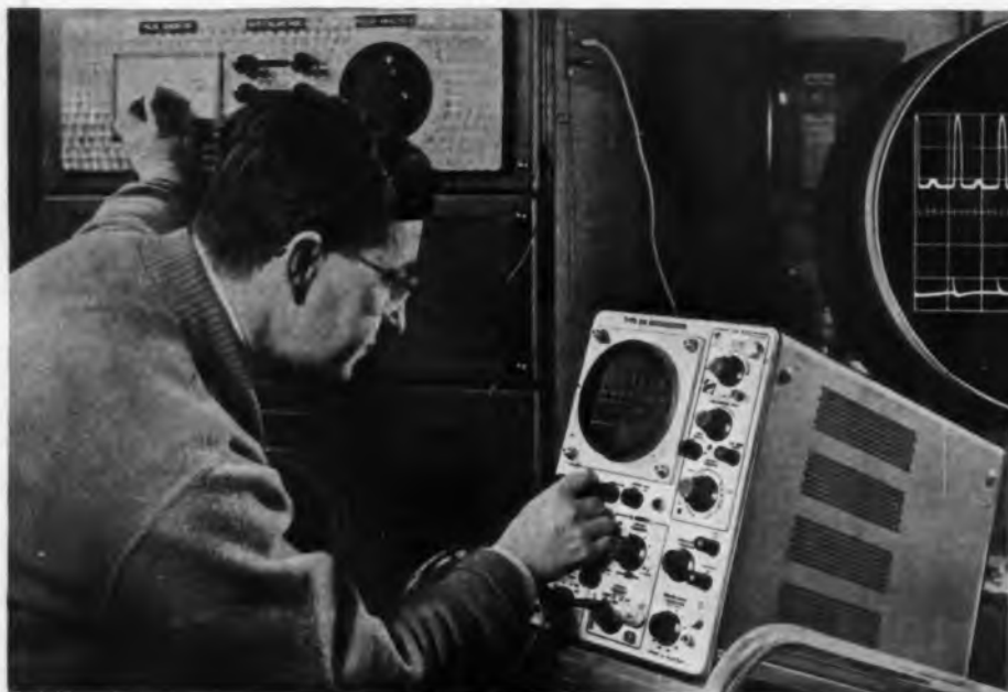
Adjusting pulse width and height (of welding signal) from newly developed Welding Control apparatus developed by MAXIM CONTROLS COMPANY, Portland, Oregon. By observing the dual-trace display on the Tektronix Type 516 Oscilloscope, the Project Engineer easily checks a welding gate output (lower trace) with respect to the trigger pulses (upper trace) and quickly notes any variations.
