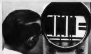
Every Spiral Accelerator gun is inspected on a high-magnification optical comparator for spacing and dimensions.
