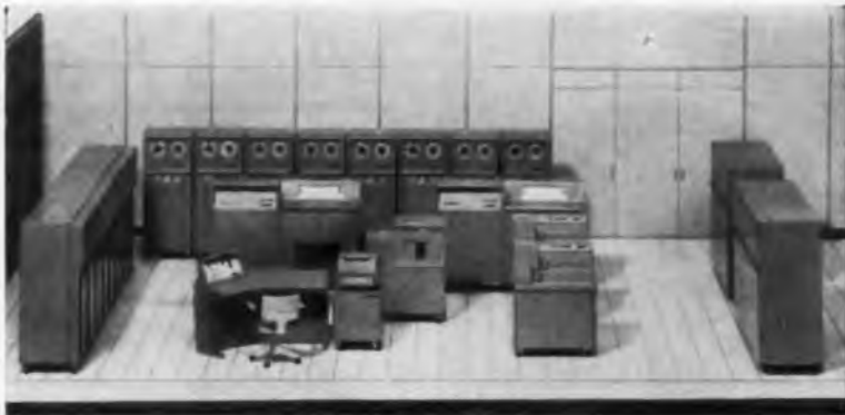
Fig. 3: The functional inter-relation of components in the system. Components may be deleted to form a system tailored to any size application.
