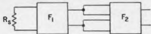
Fig. 3: The front end insert is assumed to have a flat passband, wide enough to cover both "signal" & "image" channel in the conventional superheterodyne. It can enhance or degrade sensitivity.
