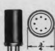
S-5207 Pin Connection Pins #1 and #6 are A.C. (Anode) Pin #7 is Pos. (Cathode) Replacement for 6X4, 6063, 6202.
