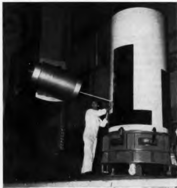
Polaris missile section set up for radiographic examination with new 10,000,000 volt linear accelerator. Varian Associates made the machine for the U. S. Naval Ammunition Depot, Concord, Cal.
