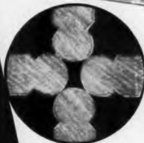
Microphotographic view of Methode Printed Circuit "FORK" CONTACTS
