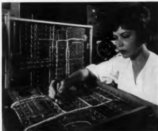
Technician checks Hughes Aircraft's "vocoder" which compresses voice by ignoring redundant sounds. This narrows the bend width enabling a tenfold increase in channel capacity. Electronic tone generators reconstruct the speed at the receiving end.
