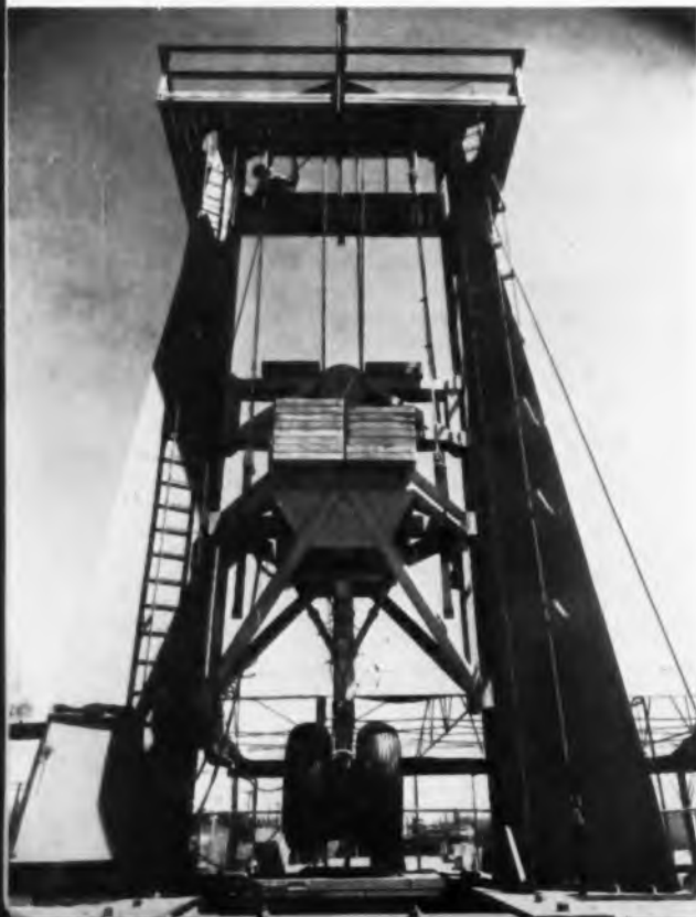
Fig. 1: Captive landing gear drop test using gages for detecting load magnitude and distribution of loads during 1/10 sec. loading.
