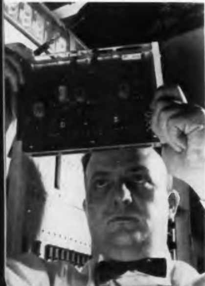
Engineer holds typical computer flip - flop card used in the Dig-itape system which electronically controls machine tools.
