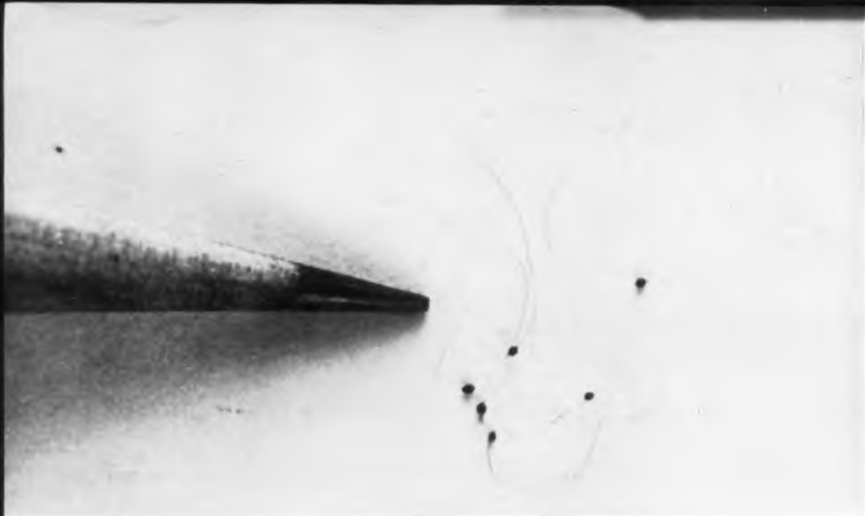
Fig. 1: Unmounted glass-coated bead thermistors used in the space respiratory gauge have a diameter of 0.014 inch.
