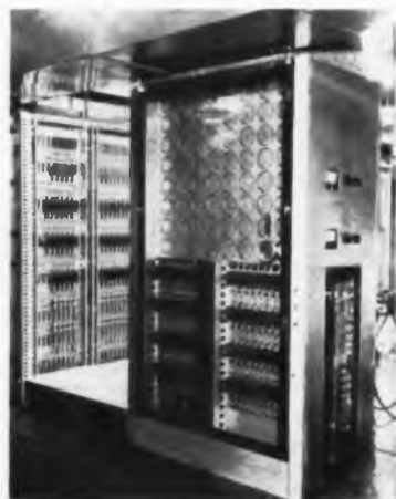
Rice Institute designed and built their own computer. The work is being financed by the Atomic Energy Commission and Shell Development Co. Shown is a view of the barrier-grid tube memory with the arithmetic unit shown in the background.
