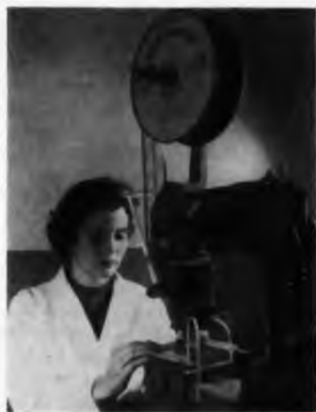
Automatic assembly insures better reproducibility. This "machine-gun" staples semiconductors into circuits, eliminating hand work.
