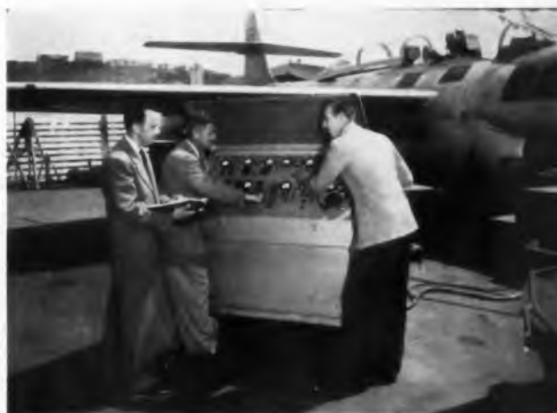
Using special test equipment, engineers check out electronic control system installed in an all-weather interceptor at Culver City, Calif.
