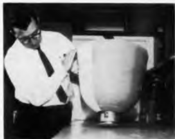
A General Electric technician displays the space radiation measurement vehicle dropped 7 miles into the ocean. Vehicle is called nuclear emulsion recovery vehicle (NERV). Drop was made to test vehicle's recovery system and its survival capabilities.
