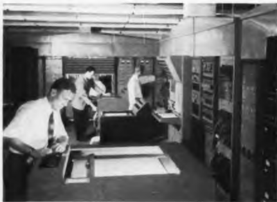
Recorder in foreground (above) traces reaction of plane equipped with electronic controls as engineers "intercept" a simulated enemy bomber. The "seek-find-and-kill" control system (right) is shown with a typical interceptor in which it is installed.
