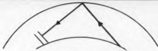
Fig. 6a: Static interference and man-made signals, reflecting from the ionosphere, may enter the beam of receiving antenna.
