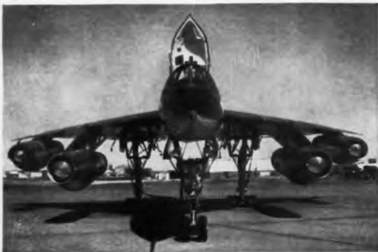
The B-58 Hustler, America's first supersonic bomber, is now in production for the U. S. Air Force at the Fort Worth, Texas, Plant of the Convair Division of General Dynamics Corporation. Carrying a crew of only three, the B-58 is designed to operate at altitudes above 50,000 feet and is powered by four General Electric J79 turbojet engines.
