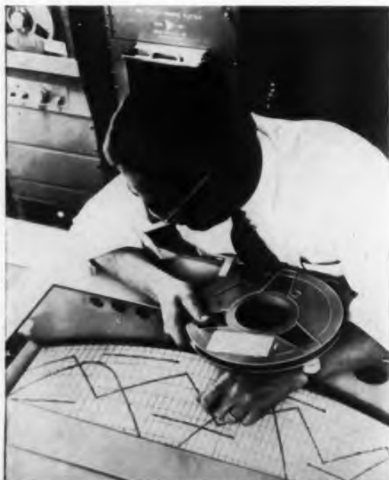
Computer-coded digital information on a 2400-ft. reel of magnetic tape can be translated into 500 pages of neatly stacked, graphed, printed, or printed-and-graphed data in just eight minutes.
