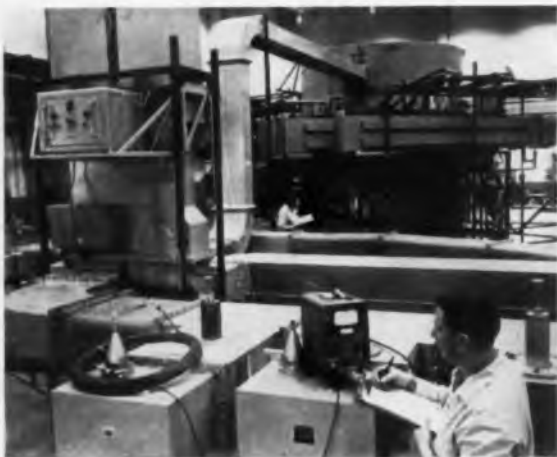
(Above) Electron Probe Duplexers being tested in GE's Syracuse lab. (Below) Transmitter Power Amplifiers being readied for testing in the same lab. Amplifiers are made by Continental Electronics Manufacturing Co. They provide power for the surveillance radar subsystem. Radio Corp. of America is the prime contractor.
