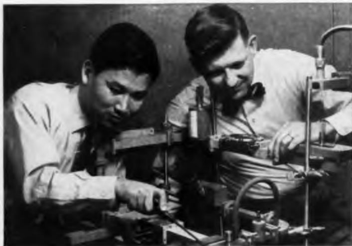
At Bell Laboratories, M. Uenohara (left) adjusts his reactance amplifier, assisted by A. E. Bakanowski, who helped develop first suitable diode. Extremely low "noise" is achieved when certain diodes are cooled in liquid nitrogen.
