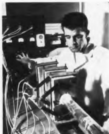
At Hughes plant technician adjusts oven temperature in "growing" germanium crystals.
