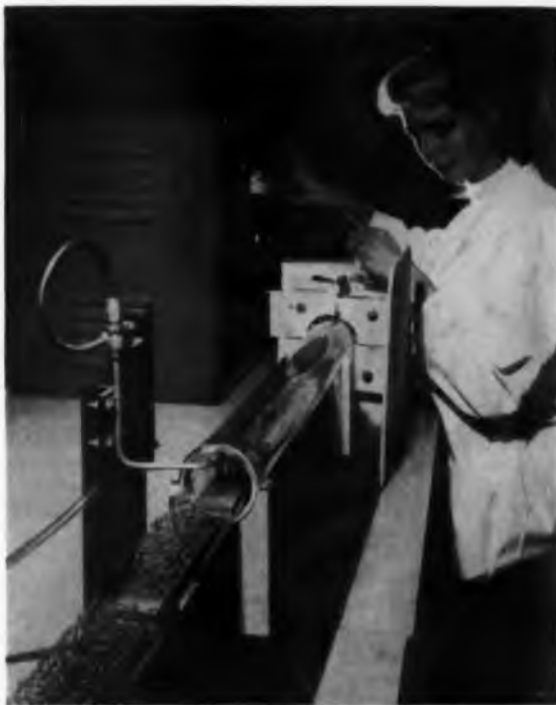
Semiconductors were by-product of military development program at Hughes. Here moving belt of partly-assembled semiconductors is guided into electric heating coil. Heat insures good connections.
