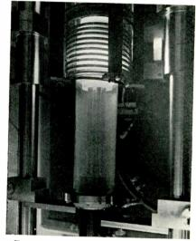
Technique developed by Knapic Electro-Physics, Inc., Palo Alto Calif., simultaneously grows silicon and germanium monocrystals by a modified Czochralski technique. Shown are four ½ in. dia. crystals growing simultaneously.
