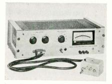
for full scale meter deflections. Bandwidth is dc to 10 KC on the 2.5 mv range, rising to 50 KC on the 1000 my range. Keithley Instruments, Inc., 12415 Euclid Ave., Cleveland 6, Ohio. Circle 199 on Inquiry Card
