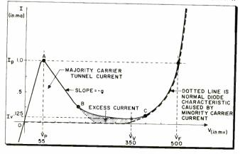
a high current, low voltage device. Further, it has a large negative conductance joining the two regions of large positive conductance. Fig. 1 shows a typical characteristic.
