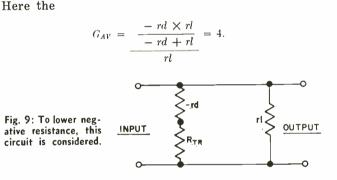
Adding 48.5 ohms  $(R_{tr})$  in series with -rd yields a total negative resistance of 48.5 + (-200) =-151.5. The resulting gain is now approximately equal to
