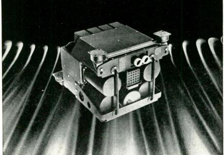
• AiResearch Central Air Data Computer for North American's A3J, Navy's first weapon system, provides information dealing with bombing. navigation, engine inlet control, radar, automatic flight control and cockpit instrumentation.
