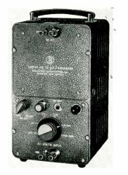
shunted by 15  $\mu\mu f$  to 25  $\mu\mu f$  depending on range. Output is a linear function of input voltage within its range. Ballantine Laboratories, Inc., Boonton, N. J.
