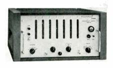
0.00003% ±0.1 CPS. Input impedance is 1 M ohms to 10 MC, 100 ohms above 10 MC. Berkeley Div., Beckman Instruments, Inc. Booth 3416. Circle 264 on Inquiry Card
