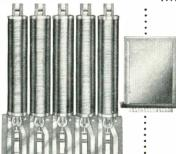
Ten CLAREED switches, mounted in line on a printed circuit board with five magnetic coils. This assembly can then be enclosed in the flat, rec-tangular container or it may be coated with "Skin-Pack," a tough vinyl plastic, and mounted directly into your equipment.
