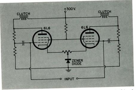
Fig. 2: Schematic shows the hysteresis clutch field coil amplifier.
