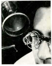
"Solid State Ionization Chamber" is smaller than the head of a pin. Developed by Hughes Aircraft Co. Labs at Los Angeles and Newport Beach, Calif., it measures the number and energy of atomic particles. It uses "doped" silicon which emits a measurable pulse when struck with a charged nuclear particle.
