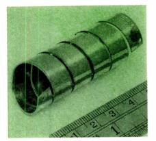
Fig. 29: Deflection plate used in the DuMont travelling w a v e deflection cathode ray tube.
