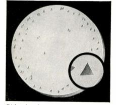
Dislocation density, Knapic silicon mono-crystals: Crystal diameters to  $\frac{3}{6}'' - None;$  $\frac{3}{8}''$  to  $\frac{3}{4}'' - less$  than 10 per sq. cm.;  $\frac{3}{4}''$  to  $\frac{1}{4}'' - less$  than 100 per sq. cm.;  $\frac{1}{2}''$  to  $\frac{2''}{4}''$ -less than 1000 per sq. cm.
