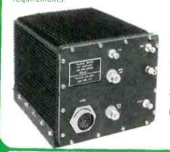
RECEIVER Frequency range: 2825-2925 MC/Sec. Stability: ±2MC/Sec. Triggering sensitivity: - 40 DBM Interrogation: (a) Single 1 microsecond pulse (b) Double 1 microsecond pulses spaced 3 microseconds Interrogation rate: 100-1500 cycles per second TRANSMITTEP
