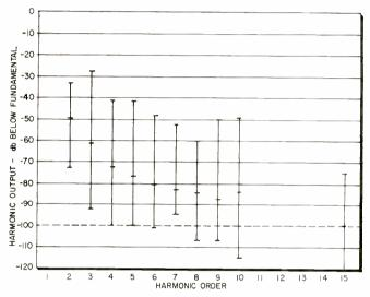
Fig. 4: Normalized harmonic emissions. Line length represents range of values and mark near line center is the mean value.
