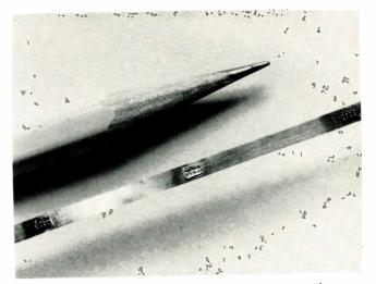
Fig. 8: Ribbon bearing multiple junction systems on germanium crystal produced by dendrite process. Three systems are shown on ribbon.
