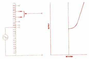
Fig. 6: The voltage step-up feature is used to generate the secant function. The taps are located in the unexcited portion of the transformer so the output voltage ratio will always be greater than one.
