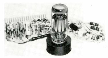
This Beam-X counting module uses only 56 components. All transistor module would require 146. Unit handles 110 KC counting frequency.
