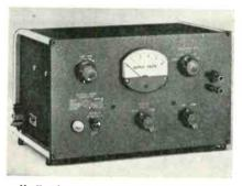
rolloff above 30 KC, the 500 KC setting a low-pass filter that rolls off above 500 KC, and the 5 MC setting a peaking network that compensates for the drop in noise output from the gas tube at high frequencies, so that a good spectrum can be obtained at 5 MC. Also featured is a built-in 80 db attenuator to provide metered outputs from over 3 v. down to below  $30\mu$ v. General Radio Co., West Concord, Mass.
