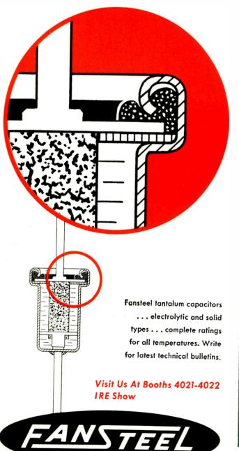
Over 10 years of laboratory testing and millions of applications in the field prove that Fansteel's patented shoulder and curl design provides *the best method of sealing* a tantalum electrolytic capacitor.
