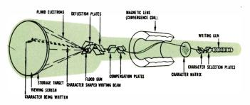
Fig. 16: Arrangement of elements in the Typotron, a display storage tube manufactured by Vacuum Tube Prods. Div., Hughes Aircraft Co.
