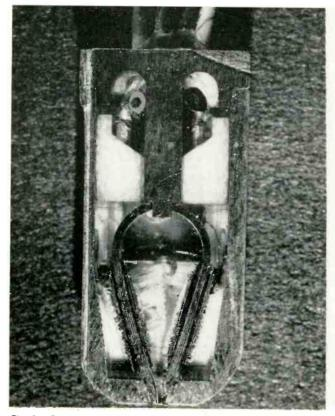
Fig. 1a: Cut-away view of the high resolution magnetic head.
