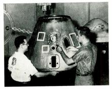
General Electric missile re-entry vehicle is equipped with instruments for measuring meteor sizes and electrical energy in space. J. Frissora of Geo-Sciences, Inc., Alamagordo, N.M., points to his self-designed membrane detector. It measures size of meteors by escaping gas. Extended ears are for measuring ion densities and potential of vehicle.
