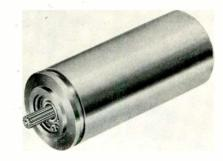
stall. Tachometer generator has 26 v RMS, 400 CPS rated input voltage and 0.26 v RMS output voltage at 1,000 RPM. John Oster Mfg. Co., Avionic Div., 1 Main St., Racine, Wis. Circle 211 on Inquiry Card
