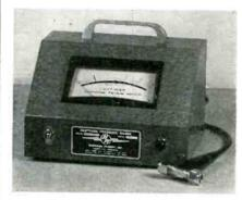
scale range is 0 to 0.01 in.  $H_2O$ . Detects differences as small as 0.0001 in.  $H_2O$ . Hastings-Raydist, Inc. Booth 3807.
