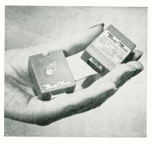
Total requirement is 20 vdc at 5 ma. Other characteristics include: input ranges — 1 v. total (min.) — 5 v. total (max.); input impedance — 100,000 ohms per v.; linearity — 0.5%; stability — 1%; temperature range — 25° to 85°C; operating environment —  $\pm$  25g. Bendix-Pacific Division, Bendix Aviation Corp., 11600 Sherman Way, North Hollywood, Calif.
