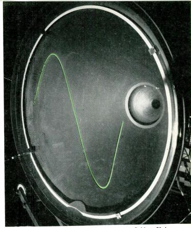
Fig. 2: Trace apparently suspended in mid-air on a DuMont 21 in. tube using a transparent phosphor. Used when ambient light is high. visual output. Under electronic output, we have a subdivision into single gun tubes and dual, or multigun tubes. In single gun tubes the one gun is used for both writing and reading. In dual gun tubes the second gun may be located either at the same end of the bulb as the writing gun or on the same axis at the other side of the storage surface.
