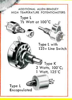
This new Allen-Bradley potentiometer—the Type L—is especially designed to solve problems associated with high ambient temperatures and space conservation. Although extremely compact—0.5 inch in diameter —the Type L control has a conservative rating of 0.5 watt when operating in an ambient temperature of 100°C. And, it provides reliable performance when operated at a temperature of  $150^{\circ}$ C—under "no load" conditions. (See graph at right.)
