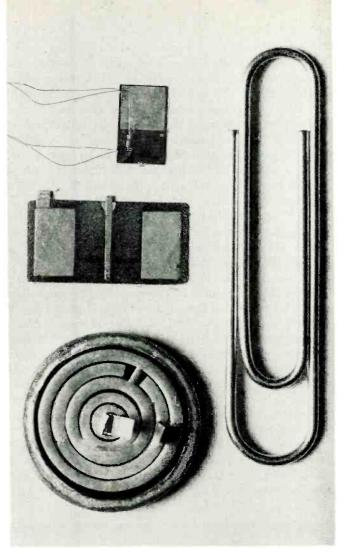
Fig. 2: Three function blocks representing subsystems: (top) a twostage video amplifier; (center) a free running multivibrator; and, (bottom) the device with the concentric arcs, an audio amplifier.
