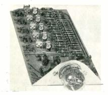
puts. Relays and tubes are eliminated. No preventive maintenance required. It activates a cold-cathode decimal display equivalent to a "Nixie" tube. Filamentary projected readout equivalent to IEE Alpha-Numberic unit available. A variety of 4 bit codes can be converted. Hermes Electronics Co., 75 Cambridge Pkwy., Cambridge 42, Mass.
