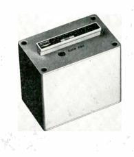
meets MIL-E-5272B Procedure III. It handles signals as low as 0 to 10 mv and as high as 250 mv. Under max. gain, an input signal of  $\pm$  10 mv will produce output signals of  $\pm$  5 v. Carrier rejection is 60 db or greater below max. output. Operating power is +20v. at 25 ma  $\pm 5\%$ . United Electro-Dynamics, 200 Allendale Rd., Pasadena, Calif.
