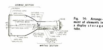
Fig. 15: RCA's direct view display storage tube. Like those of other manufacturers, it is used where a bright, non-flickering display of stored information is dewriting sired after
