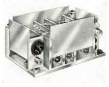
put is 2 to 6 w at 215 to 260 MC. Carrier stability is 0.005%. Telechrome Manufacturing Corp. Booth 3612.
