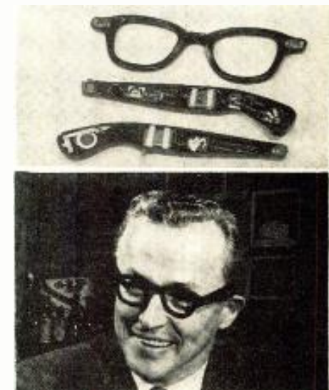
Amplifier components are concealed in frames
