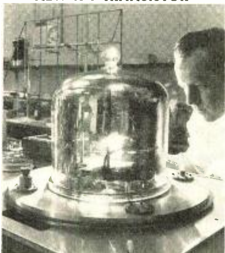
New germanium diffused-base transistors being manufactured at Bell Labs. Frequency cutoff of transistors is between 500-600 MC
