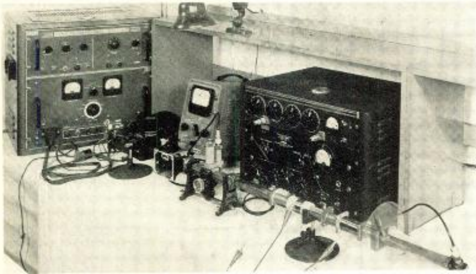
Fig. 1: Equipment for measuring Faraday rotation. Microwave energy from klystron signal source (l) enters wave guide containing two ferrite sections which rotate the propagation mode. Barretter (r.) feeds output energy to receiver
