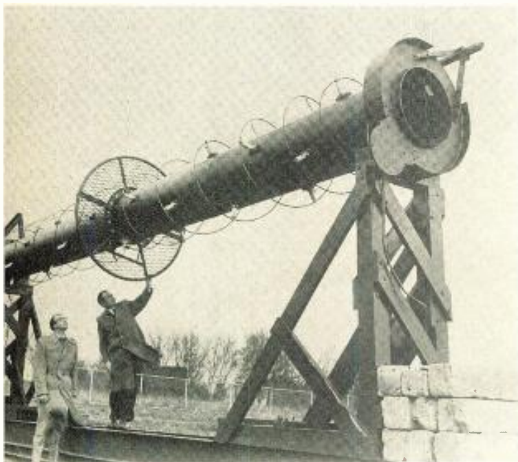
G-E engineers call this "the simplest TV broadcast antenna that you can hoist to a tower top." Designed for operation on Chs. 7 through 13, it has only three feed points as compared to the usual 16 points of the conventional antenna. The 3,500 lb, all-steel antenna has a gain of four, and will reportedly permit doubling the power of present stations.
