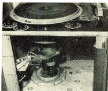
Turntable modification prevents closing of brake on clutch from spoiling cued-in start
