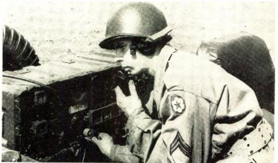
Reportedly four times more powerful than the WW II-Korean models, the new versatile AN/GRC-19 functions both as a 100 wpm radio teleprinter and as a radiotelephone. It is designed for mounting in parachute-dropped vehicles and tanks. The unit was developed jointly by the Signal Corps Engrg. Labs and Collins Radio Co.
