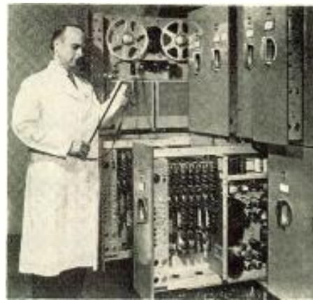
J. Wesley Leas, chief engineer of the "Bizmac" project — the $4-million electronic data processing system bought by the U. S. Army from RCA — examines magnetic tape. More than 2,500,000 digits can be stored on single tape. "Bizmac" will handle inventory control at the Ordnance Tank-Automotive Command in Detroit.
