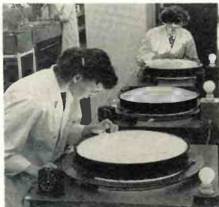
RCA's 21AXP22's round metal three-gun color tubes being tested in lighthouses in the Lancaster Tube Div. plant See page 158 for additional details.
