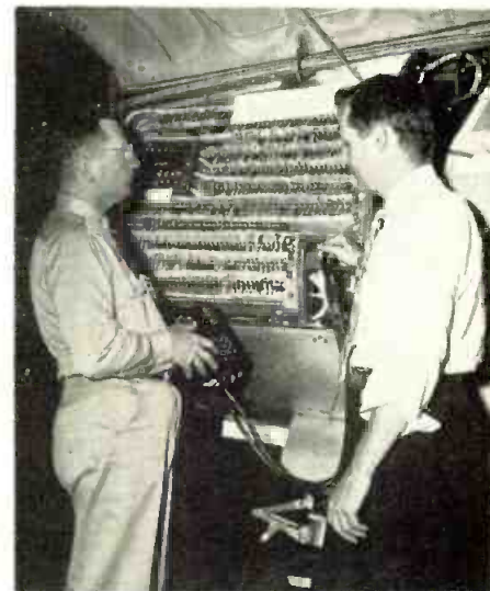
Max Beers, Sperry Gyroscope project chief, and Lt. Col. J. P. Grant check out remote beeper control system for pilotless jet aircraft
