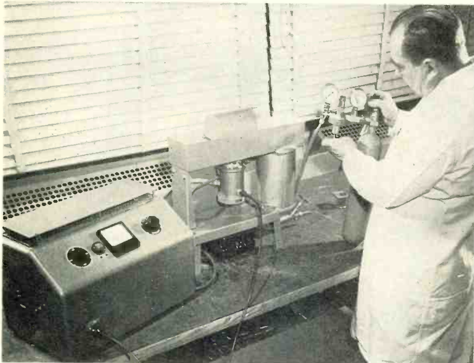
Curtiss-Wright's new ultrasonic parts washing machine cleans metal objects such as fuze movements and delicate foils. Objects immersed in solvent solution have grime loosened by cavitation and degassing. Power output of 800 kc units range from 200 to 10,000 watts. Either quartz or magnetostrictive transducers are employed. Cost of ultrasonic generator and head is about $1250
