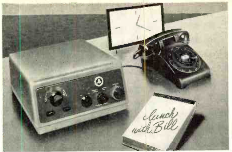
TELEPHONE ANSWERING. When you aren't there, the automatic telephone answering set takes over, delivers previously dictated message in your voice, records caller's reply and plays it back to you at your convenience.
