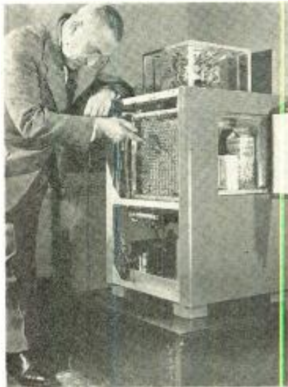
Nils Lindenblad of RCA Labs. inspects electronic cooling system believed to be first of its kind to achieve practical freezing temperatures. Operation is based on "Peltier effect," described on page 110
