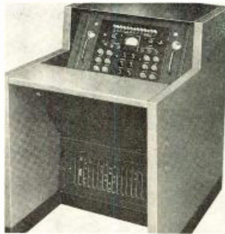
Fig. 12: Master console, including camera control panel and processing amplifier units
