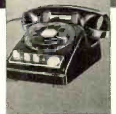
"HANDS-FREE" TALKING. Telephone set base has a built-in microphone — you talk without picking up handset. Tiny desk speaker amplifies the distant voice so that several persons in a group can listen to the conversation. For privacy, you lift the receiver, automatically shutting off the microphone and speaker. Small amplifier, not visible in the picture, furnishes power.
