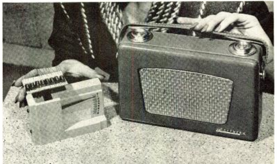
An eight-transistor portable radio which operates for 500 hours using power solely from four standard flashlight cells will go on sale March 1 for $79.95. The 5-lb. unit made by Raytheon Mfg. Co. measures 2-5/8 in. thick, 6-3/16 in. high, and 9-3/16 in. wide. By using special mercuric oxide batteries, which cost five times as much as ordinary type, 2500 hours of performance, the equivalent of five years of operation, can be obtained. Five CK760 transistors are used in converter, oscillator, i-f and detector stages. Other three units being weighed in photo are CK722's for audio stages. AVC, ceramic ferro-magnetic rod antenna and 3-1/2 in. speaker are other features incorporated in radio
