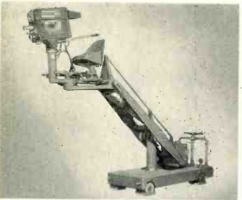
HOUSTON-FEARLESS TC-1 CRANE raises camera to extremely high and low positions. Permits "fluid motion" shots. Foot-operated panning.
