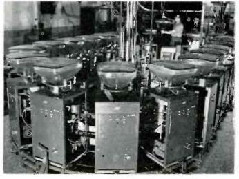
Completion of automatic aluminized TV picture tube facilities enables additional output of 25,000 more units per month. Photo at left shows new settling room under one man centralized control. At right new equipment for automatic in-line aluminizers are seen.
