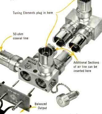
The Type 874-UB Balun is a unique device for connecting from balanced to unbalanced systems over a wide 54 to 1000 Mc range. The balanced to unbalanced transformation is obtained by using a semi-artificial, half-wave line made up of two sections of 50-ohm coaxial line and two shunt tuning elements.
