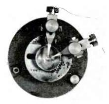
Fig. 5: Photo of specimen mounting jig
