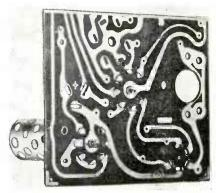
which enables printing jumpers to connect different pin positions. Static load tests indicate that, when properly dipsoldered in a multiple hole pattern in a printed wiring panel, the socket will withstand a force of 10 times normal tube withdrawal force. Available in 7 or 9 pin types. Methode Mfg. Corp., 2921 W. Churchill. Chicago, III.—TELETECH & ELECTRONIC INDUSTRIES. (Ask for 12-27)
