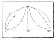
Fig. 2: Low-current curves are clue to inaccuracy. Copper oxide rectifier vs ac sine current; B) Sinewave; C) rectifier vs ac sine voltage
