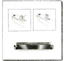
two terminal styles; (1) a slotted eyelet for soldering up to three No. 20 AWG cable wires per contact (2) a plain terminal to permit wire wrapping by the Western Electric Co. "Wire-Wrap" tool. Contact mv. drop is 10.5 dc at 3 amps rated current. Gold plating over silver provides low electrical resistance, corrosion prevention, and soldering ease. Winchester Electronics, Inc., Willard Rd., Norwalk, Conn.—TELE-TECH & ELECTRONIC INDUSTRIES. (Ask for 12-19)
