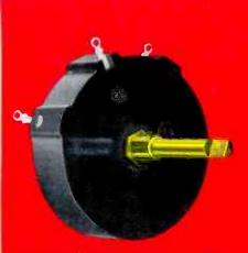
High voltage control for focus applications. Rated up to 5,000 volts DC across end terminals and 2 1/2 watts depending on total resistance. Will operate up to 15,000 volts DC above ground when mounted on insulated panel. CTS type 85.
