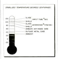
Fig. 4: Comparison of operating temperatures of various components in I-f amplifier
