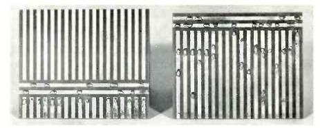
Fig. 2b: Printed wiring side of amplifier showing arrangements of breaks and solder points
