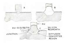
Fig. 8: Diagram of fusion mechanism
