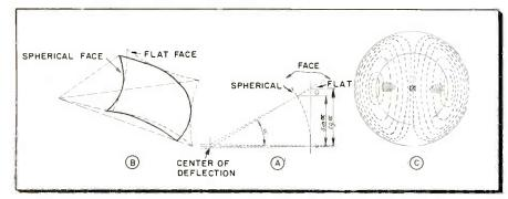
Fig. 1 (A) Spot distortion in flat-face tube with uniform field (B) Spherical and flat-face raster differences (C) Cross section of magnetic field in yoke on the neck of the picture tube
