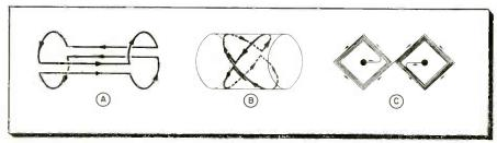
Fig. 4:(A) Usual shape coil cannot be entirely free from end-effects (B) Interlaced elliptical coils eliminate end-effects (C) Planar view of printed crossed-field deflecting coils
