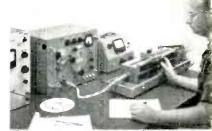
Electronics Research Engineer F. R. Zboril measures input impedance of a scale model helical antenna array used for ground tracking of missiles. Most of Lockheed's other antenna work involves advanced research studies on flush mounted antennas.
