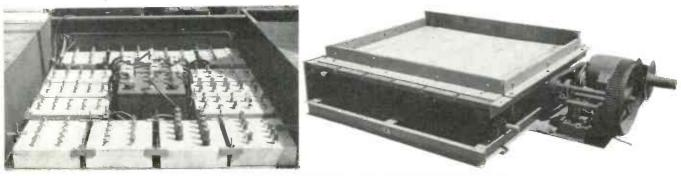
Fig. 3: (I) Method of mounting electronic chassis, Fig. 4: (r) L.A.B. package tester
