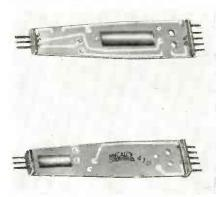
tions. The units feature molded-in inserts. The coefficient of thermal expansion of the components is close enough to that of most inserts to hold them tight over the operating ranges. The glass-bonded mica (Mycalex 410) from which the components are molded is structurally rigid and holds its hardware in true alignment. Mycalex Corp. of America, 60 Clifton Blvd.. Clifton, N.J.—TELE-TECH & ELECTRONIC INDUSTRIES. (Ask for 12-26)
