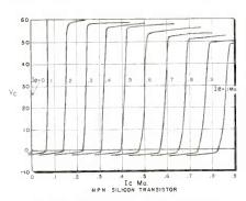
Fig. 12: Characteristic curves of fairly good silicon transistor with alpha 0.9
