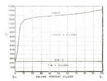
Fig. 1: Phase diagram of silicon-tin system
