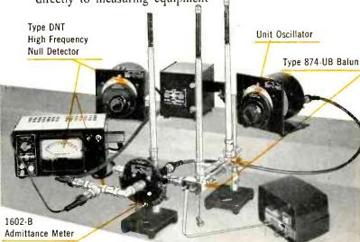
Type 1602-B Admittance Meter and Balun setup to measure admittance or impedance of converter input. One Type 1208-A Unit Oscillator supplies the vhf power, while the local oscillator in the Type DNT Null Detector Assembly beats with the Admittance Meter output to provide a 30-Mc difference frequency. This signal is detected by the new Type 1216-A Unit I-F Amplifier, also an element of the Null Detector Assembly.
