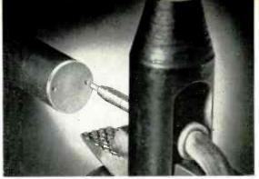
(I) Cutting a 24-pitch thread on inside wall of glass tubing having ID of  $\frac{1}{2}$  in., using right angle nozzle with 0.006 x 0.06 in. rectangular orifice. Similar helixes have been cut in ceramic tubing with 0.17 ID. (r) Prilling depression in quartz disc. Hole is 0.03 in. dia., 0.015 in. deep.
