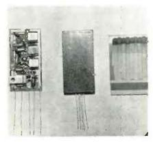
sistors. The printed unit is now available in sample quantities with solder terminals, or as a plug-in device. Size,  $\frac{6}{10}$  x 1 x 2 in. Weight, less than  $\frac{1}{2}$  oz. Input impedance. 400 to 1,200 ohms; output impedance. 120 to 2,000 ohms. Power output, 73 mw. Sensitivity, 500 µv. Power source, 28 v. dc. Plastics & Electronics Corp., 272 Northland Ave., Buffalo 8, N.Y.—TELE,—TECH & ELECTRONIC INDUSTRIES. (Ask for 12-23)
