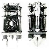
Fig. 3: (I) I-F transformer construction details, showing toroidal coil and resistors. Fig. 4: (r) View showing unit's plunger capacitor
