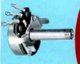
Ear mounted tandem for preset applications. Combines panel space saving features of a concentric tandem with the economy of an ear mounted unit. Available in various combinations of composition or wirewound front and rear sections. CTS type P-C2-45 with composition front and rear sections illustrated.
