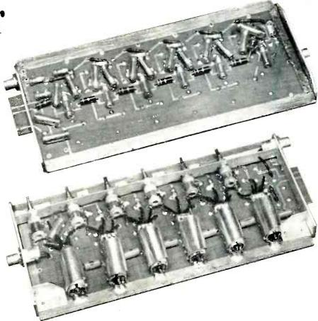
Fig. 2: (Above) Photo of both sides of seven inch unit with cover removed. Design features high reliability, simplified production and circuit uniformity. Fig. 3: (1) Cover plates are held together by sliding clips, not screws
