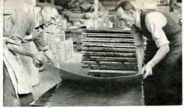
Fig. 1: Makeup sheet of foll-clad material consists of arranging laminate, adhesive (dry film in this instance) and copper foil in proper sequence. Adhesive must contact rough side of both laminate and foil for best possible bond. Fig. 2 (Right) Makeup for each sheet is sandwiched between clean smooth steel press plates. These assemblies are then stacked 5 ft. high (packs) for insertion in hydraulic presses
