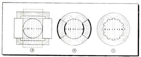
Fig. 2: (A) Using square or rectangular core is simplest way to obtain uniform deflecting field. (B) Ring core is better but requires cosine winding to restore field puniformity (C) More recent and still better approach is in castellated core
