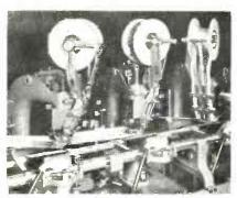
station automatically Inserting prepares, and inserts components through prepunched holes in p-w boards. Auxiliary lead straightening and belting machine facilitates components with pig-tail leads
