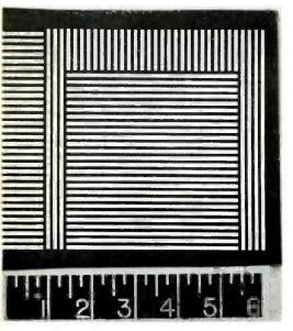
Fig. 1: Universal printed circuit board consists of pattern of wiring on one side which may be connected in a large number of combinations
