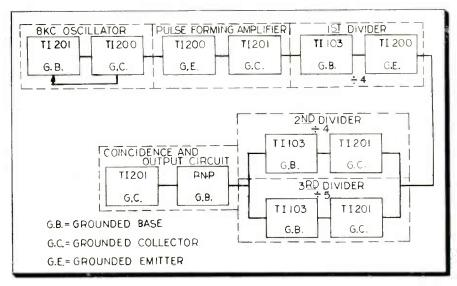
Fig. 2: Counting circuit with oscillator, dividers, pulse forming amplifier and coincidence circuit
