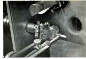
(I) Cutting a continuous spiral groove in a deposited carbon film resistor, using a straight nozzle with 0.006 x 0.06 in, rectangular orifice. Cut width is 0.007 in. (r) Cutting and shaping cylindrical crystals used in neutron diffraction. Sizes are as small as fraction of mm dia., and 1.5 cm long
