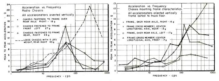
Fig. 8: (I) Acceleration spectrum of radio chassis during test. Fig. 9: (r) Acceleration spectrum of mounting frame during test
