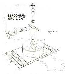
Fig. 4: Diagram of micro technique apparatus to measure lifetime degradation
