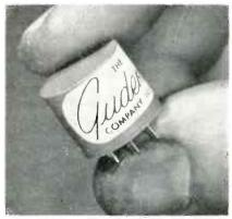
resin impregnated and molded. Operating temperature range is from  $-70^{\circ}$ C. to  $135^{\circ}$ C. The transformers surpass MILT-27, Grade 1, Class A specifications. Size,  $\frac{5}{8}$  in. diam. by  $\frac{9}{16}$  in. high. Weight, approximately 5 grams. Terminals are 22 AWG copper wire. Maximum length  $\frac{1}{16}$  in. Hi-pot test, 2,000 v. RMS. Gudeman Co. of California, Inc., 9200 Exposition Blvd., Los Angeles 34, Calif.—TELE-TECH & ELECTRONIC INDUSTRIES. (Ask for 12-17)
