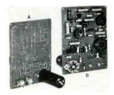
Fig. 1: Top & bottom views of printed circuit frequency standard show component arrangement
