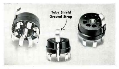
New Sylvania 7-pin Miniature Printed-circuit Sockets. Contacts and center shield are shaped so that sockets can be stacked one upon another for automatic feeding and assembly. Small slots are used on the circuit board to receive the contacts, resulting in stronger chassis construction. Only one socket assembly need be stocked since terminals can be interconnected by printing the circuit on the chassis board rather than using a metallic connector on the socket itself.
