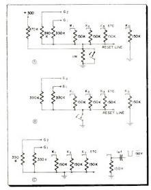
Fig. 4: Methods of accomplishing reset. (a) Positive voltage on reset line. (b) Floating reset line. (c) Grounding and negative reset
