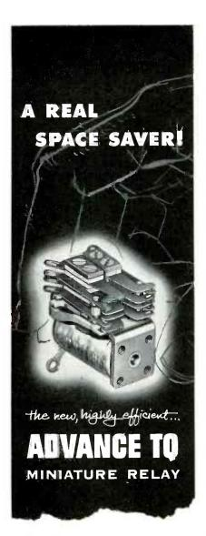
Only .94 cu. inches in size—yet it carries 3-amp. loads in the 4PDT combination. It's available up to 6PDT, and with class "H" insulation.
