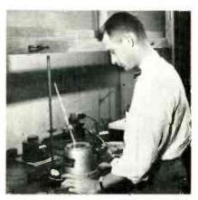
Fig. 5: Dip solder tests, One sq. in, blocks of copper clad phenolite are checked for blistering and adhesion, Usual NEMA test is 220° C for 10 seconds
