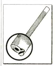
Fig. 2: Tool for fast and uniform spinning of tailored component leads on terminals
