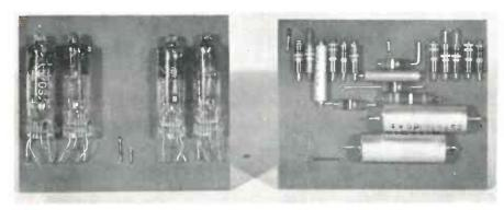
Fig. 2c: Reverse side of boards in Fig. 2b shows tubes and components connected to wiring
