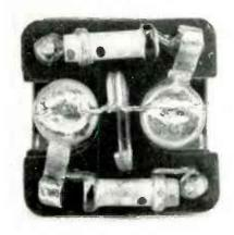
Fig. 5: Top view of i-f transformer
