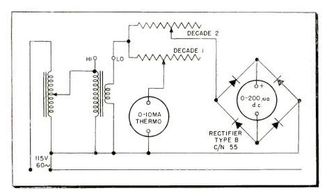
Fig. 1: Test set-up with thermo-milliammeter to obtain data on voltage doubling method
