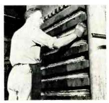
Fig. 3: Operator loads packs in 10 opening press. After one hour at 350° F and 1000 lb½/sq. in. foil and laminate are bonded
