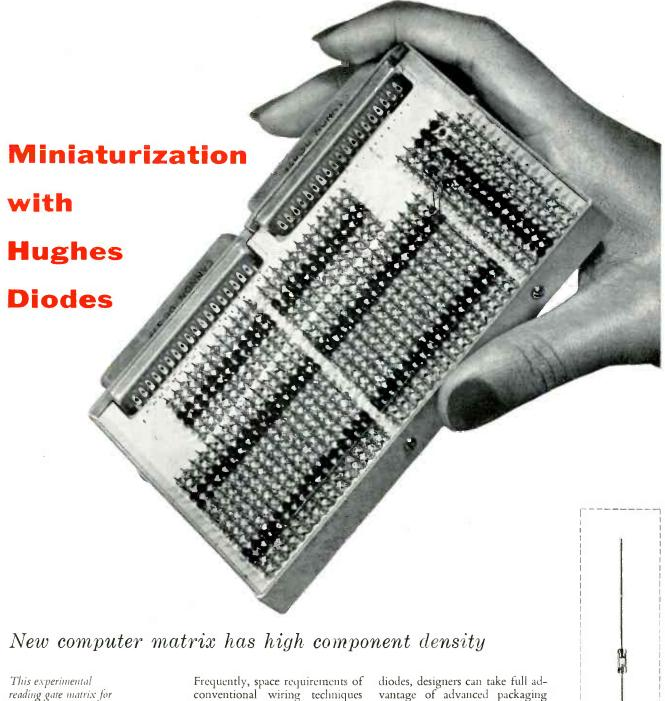
reading gate matrix for airhorne computers effectively utilizes the subminiature size of Hughes Point-Contact Germanium Diodes\*. Developed by the Miniaturization Group of Hughes Research and Development Laboratories, the unit measures 51/4 by 31/8 by 1/2 inches (excluding plugs and frame). It contains 504 diodes, 209 resistors. Average component density: 94.5 per cubic inch!
