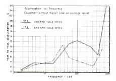
Fig. 11: Spectrum of equipment without transit case measured on package tester
