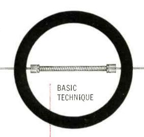
Wire element is uniformly and tightly wound on an Insulated core. Axial leads or other terminations are secured to element by automatic machinery. Insulated housing may be used or omitted.
