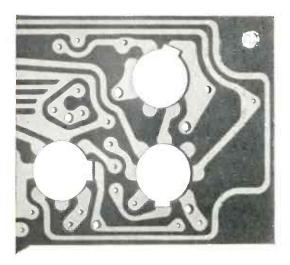
Printed Circuit Boards Printed and Accurately Punched Ready for Components.
