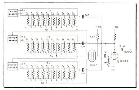
Fig. 9: Cascaded 10-count tube circuit for counting up to 1000
