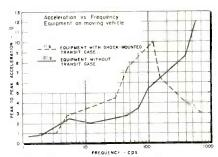
Fig. 10: Spectrum of equipment on moving vehicle with and without transit case
