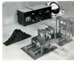
Equipment used to plot magnetic field inside deflection yokes. Note 3D field model
