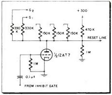
Fig. 7: (I) Reset with switch tube which cuts off when signal appears, allowing reset line to drift up. Fig. 8: (r) Similar "forced" reset switches 200 volts to line
