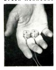
Another application of HYSOL 6000 Series Compounds, based on the new epoxy compounds, is the encapsulation for Brush Electronics Company's BK-1090 magnetic record-reproduce heads. This "Redhead" has the standard track width designed for dual track recording on 1/4" tape.
