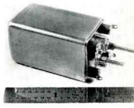
Fig. 1: Stabilized i-f transformer in can
