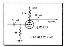
Fig. 5: Inhibit gate eliminates positive pulse
