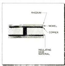
switching contacts to ride over it without bounce. The method is used in assemblies ranging from radio sets to complex analog computers. Insulated Circuits Inc., 115 Roosevelt Ave., Belleville, N.J.—TELE-TECH & ELEC-TRONIC INDUSTRIES. (Ask for 12-22)
