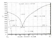
Fig. 7: Gold-silicon phase diagram
