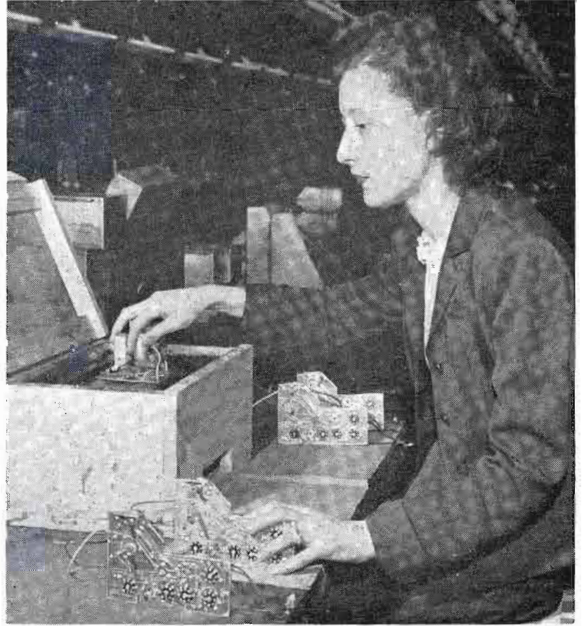
Fig. 5: Solder dip in first of two pots in double pot method
