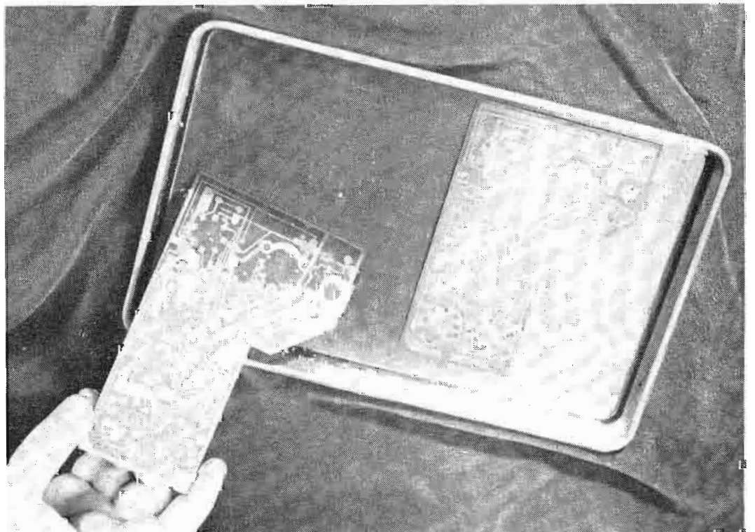
Fig. 1: Oxide removing bath prepares surface. Rinsing, drying and soldering operations follow
