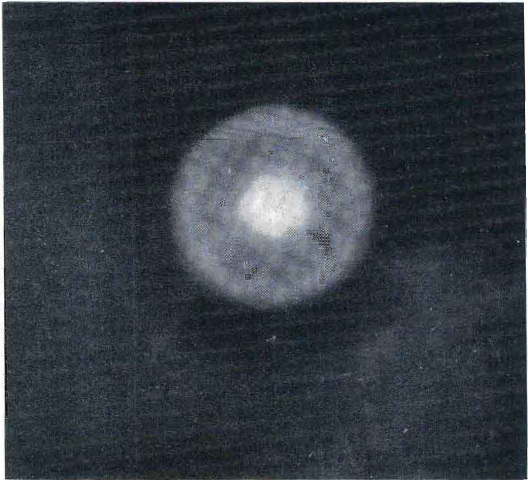
Fig. 2: Scanning spot, attendant halation rings and normal reflection
