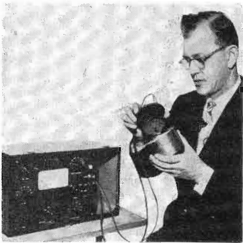
Mr. Philip E. Ohmart, inventor of the atomic battery, with a cell used for the detection of beta particles. "Aquadag" is used as an electrode
