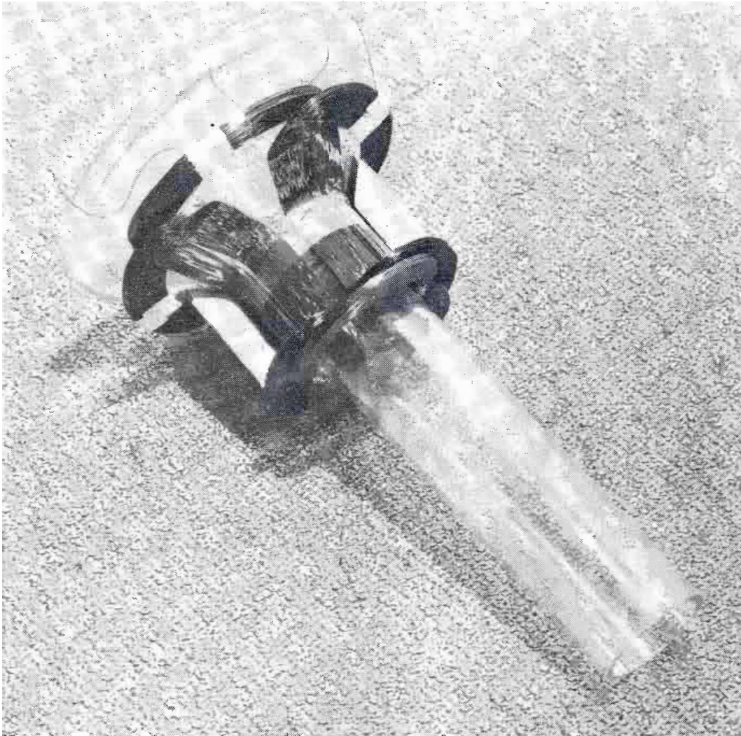
Fig. 5: Partial assembly of 90° yoke coils shows extent of coil-incline overlay on flared portion of picture tube neck funnel. Nylon housing is omitted in photograph
