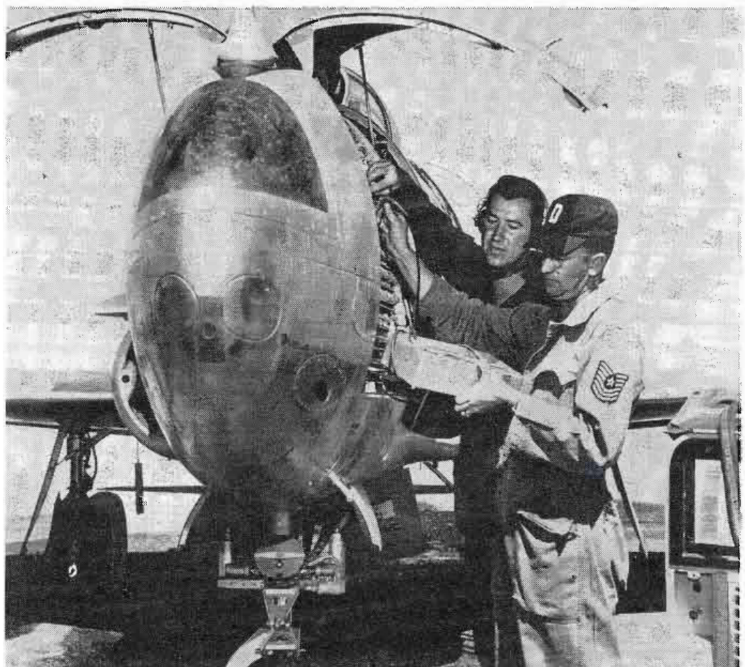
Robot controls on Lockheed QF-80 pilotless jet get pre-flight test by "beep pilots." The controls, produced by Sperry Gyroscope for the Air Force, receive beep-box radar or radar signals from two ground stations or director plane. Craft is being used in atomic bomb tests at Nevada Proving Grounds
