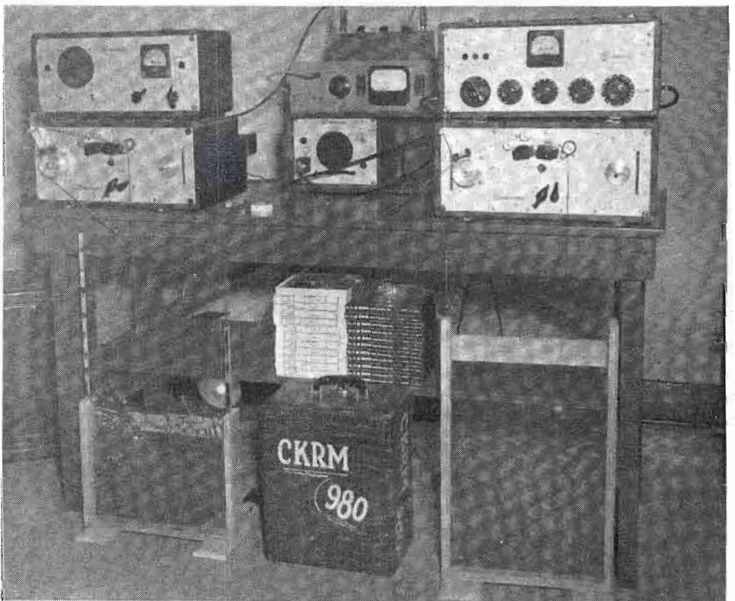
Tape delay system allowing fifteen minute delay on a two-hour program, designed by William McDonald, Chief Engineer, CKRM, Regina, Saskatchewan, Canada.
