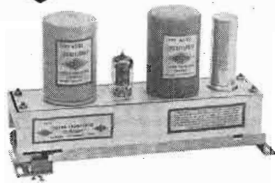
101-AX. A laboratory pre-amplifier. Uses single 12AX7 tube with triode sections in cascade. 42 and 32 db fixed gain. 80 db signal to noise ratio at maximum output. Intermodulation 2% at plus 4 dbm (using 12 kc and 40 cps at ratio of 1 to 4). Multi-impedance input and output. Feedback loop purposely does not include input and output transformers, thus allowing for complete line isolation and maximum flexibility. Complete details in Catalogue 16-C.
