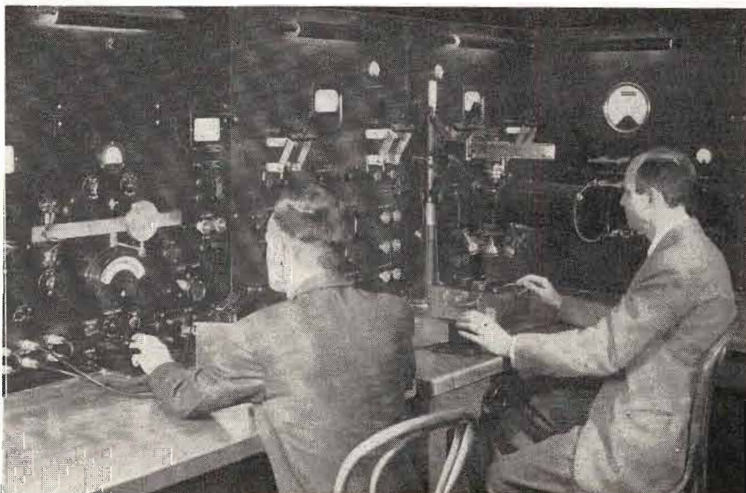
Standardization of an ac voltmeter. At left, dc voltage required to give same response in electrothermic transfer standard is being determined. Right, instrument's scale is read on projection device
