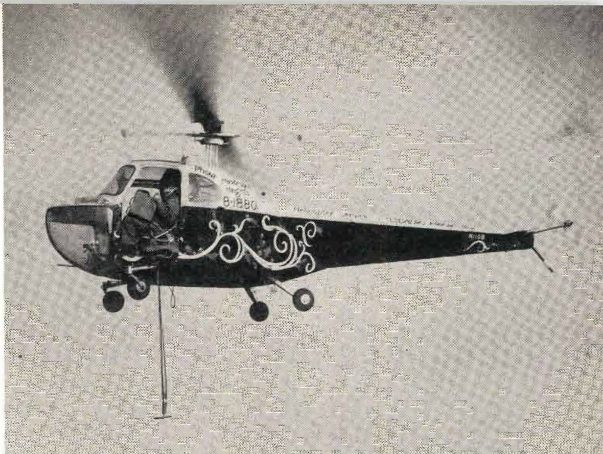
Fig. 3: Bell helicopter used in flight tests has doors removed to provide maximum ground visibility
