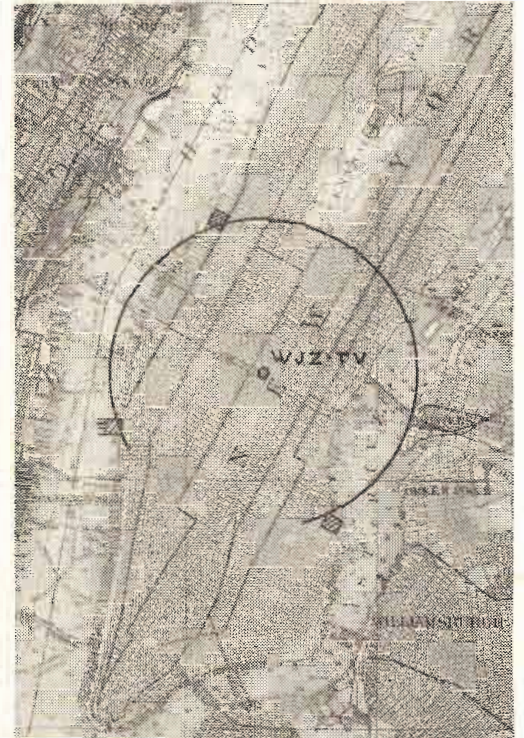
Fig. 2: Flight course of 1.4 mi. radius and 1425 ft. altitude for recording WJZ-TV field
