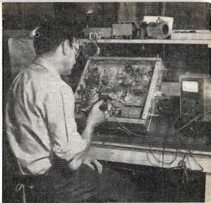
Making high voltage and resistance check on finished chassis
