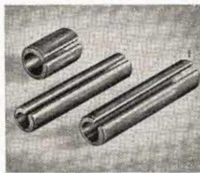
Rollpins are supplied to specified lengths with chamfered ends. Available from stock in diameters from 5/64 inch to 1/2 inch in Carbon Steel and Stainless Steel.
