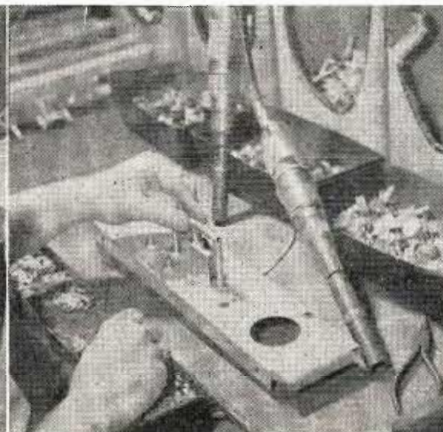
9 After airgun has tightened control lockwashers and nuts to panel, switch subassembly is added. Note jig to steady control shafts
