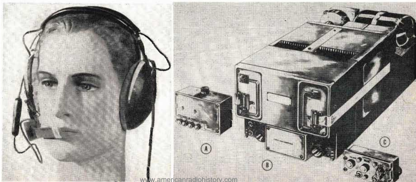
(Left) Photograph illustrates new combination dynamic noise cancelling microphone and dynamic headset. (Right) A subminiature command transceiver showing channel set-up box at left, transmitter-receiver in center and the pilot's control box at right
