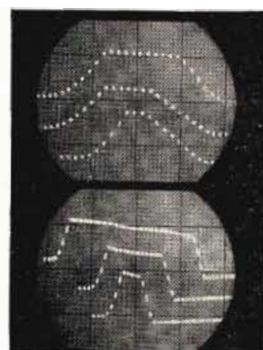
3. MULTIPLE EXPOSURE PRE-SOLARIZATION. Here, by making 3 successive exposures on each half of the print, the engineer was able to record performance of a camera shutter at its 1/100, 1/200, 1/400 second (upper) and 1/25, 1/50, and 1/100 second settings (lower). "Pre-solarizing," the process of pre-exposing the print with the trace off the screen, made it possible to record the high writing speeds involved.
