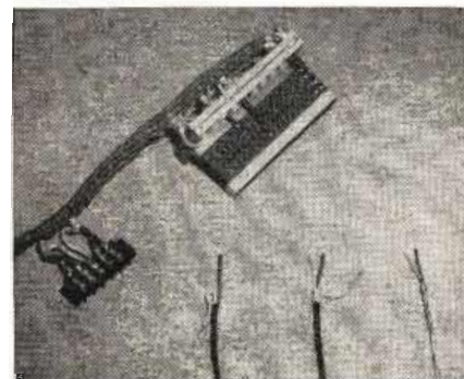
Alternative connections to WE 100B block, and method of finishing-off by pulling wires through shield to form ground leads
