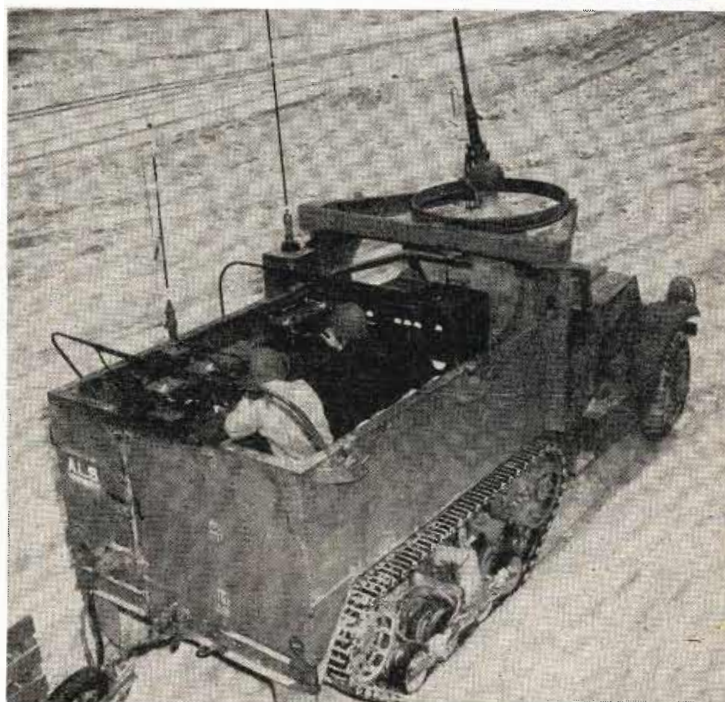
Interior SCR-299 on half-track mount used in Air Liaison Communication. Note 60-caliber machine gun for anti-aircraft protection.
