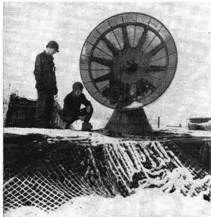
Minor repairs being made on parabolic radar antenna used by antiaircraft outfit with U. S. Third Army in Luxemburg.
