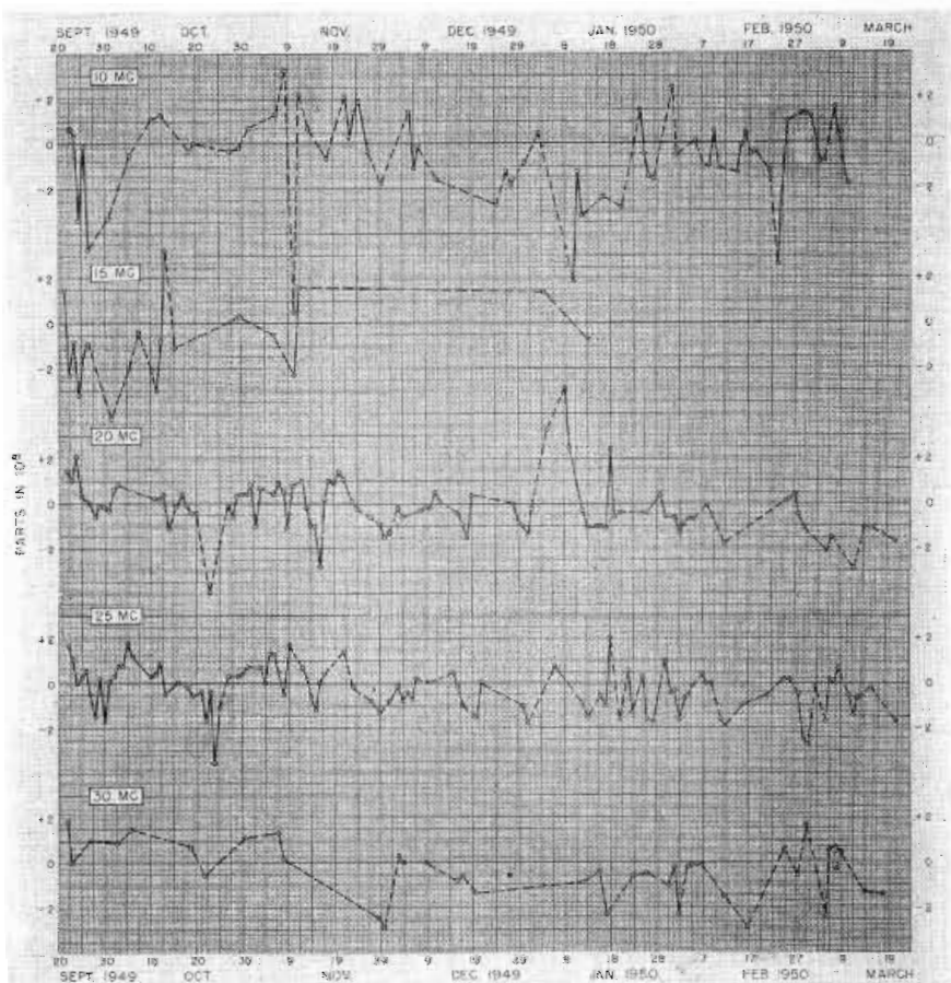
Fig. 2: Daily frequency deviation recordings of WWV, made at WWVH, Maui, T.H., note superiority of higher frequency transmissions which produced more consistent results
