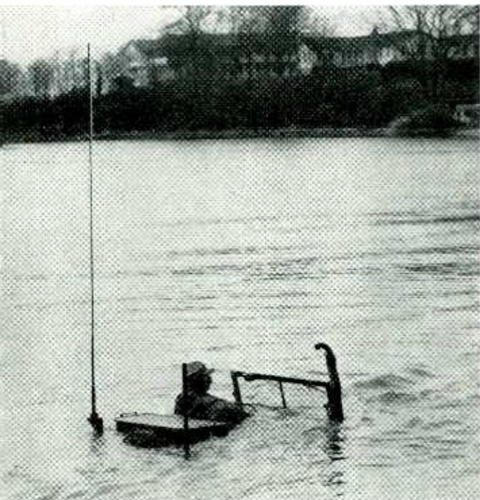
Both radio and jeep operate submerged as well as ever, even with water up to the driver's shoulders. This official U. S. Marine Corps photo shows one of the new units being developed for the Marine Corps Equipment Board
