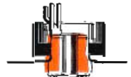
Silicone bushings and plastic cups used with capacitors 660-v a-c, or 1500-v d-c and lower.
