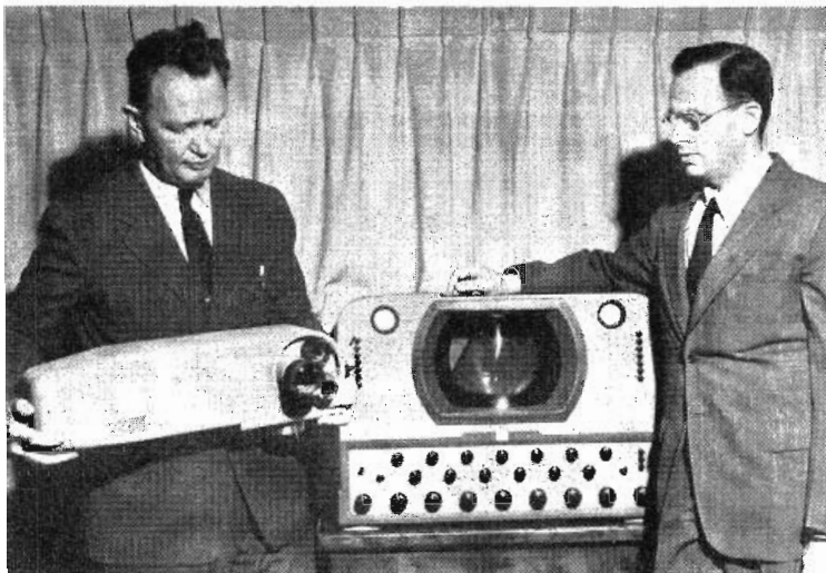
J. Reeves (left) and Dr. Peter Goldmark demonstrating the new CBS color camera and control unit. The equipment shown is all that is required to put a color picture on the air, plus, of course, a transmitter. The unit on the right is a complete sync. generator and 12-inch color picture monitor. The camera is remotely controlled and uses a standard image orthicon.
