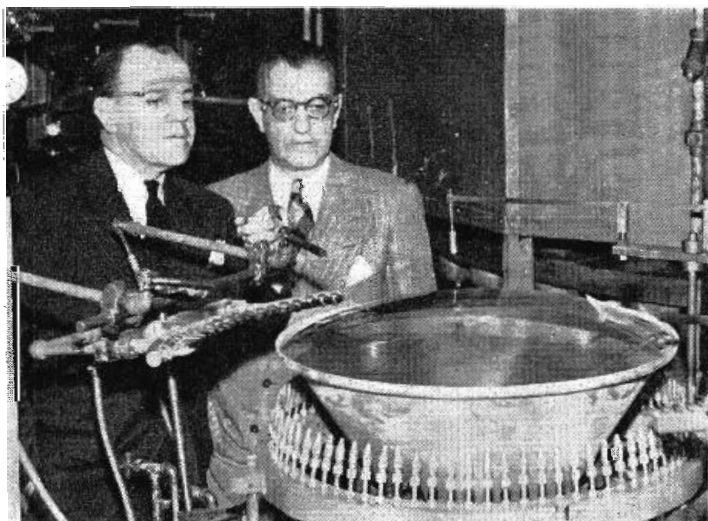
J. M. Lang and Dr. W. R. G. Baker inspect G.E.'s new 24-inch television picture-tube, shown mounted on a glass-to-metal cone-sealer. Production of giant tube will get underway this Fall.
