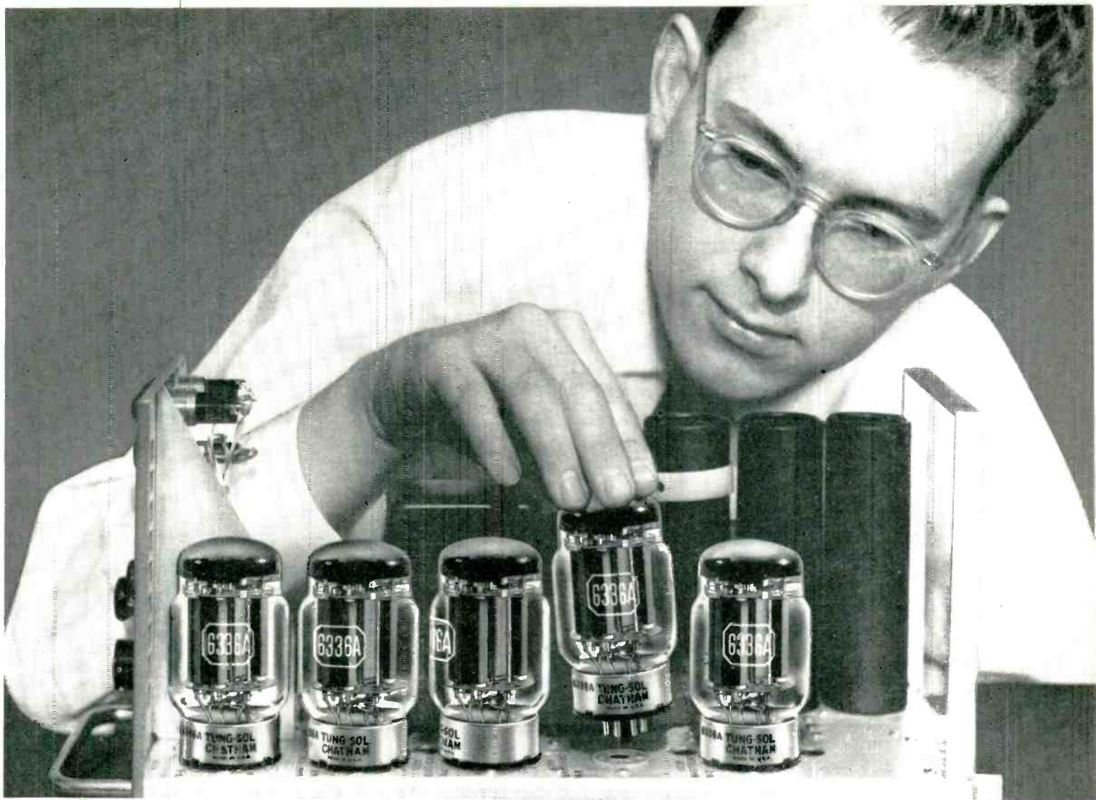
Engineer A. M. Darbie installs a Tung-Sol/Chatham 6336A twin power triode in a Harrison Labs 2B regulator, part of a 200B high current power supply. Superior power handling ability of the 6336A lets Harrison Labs offer the regulator with a 5-tube complement in addition to a 7-tube model.
