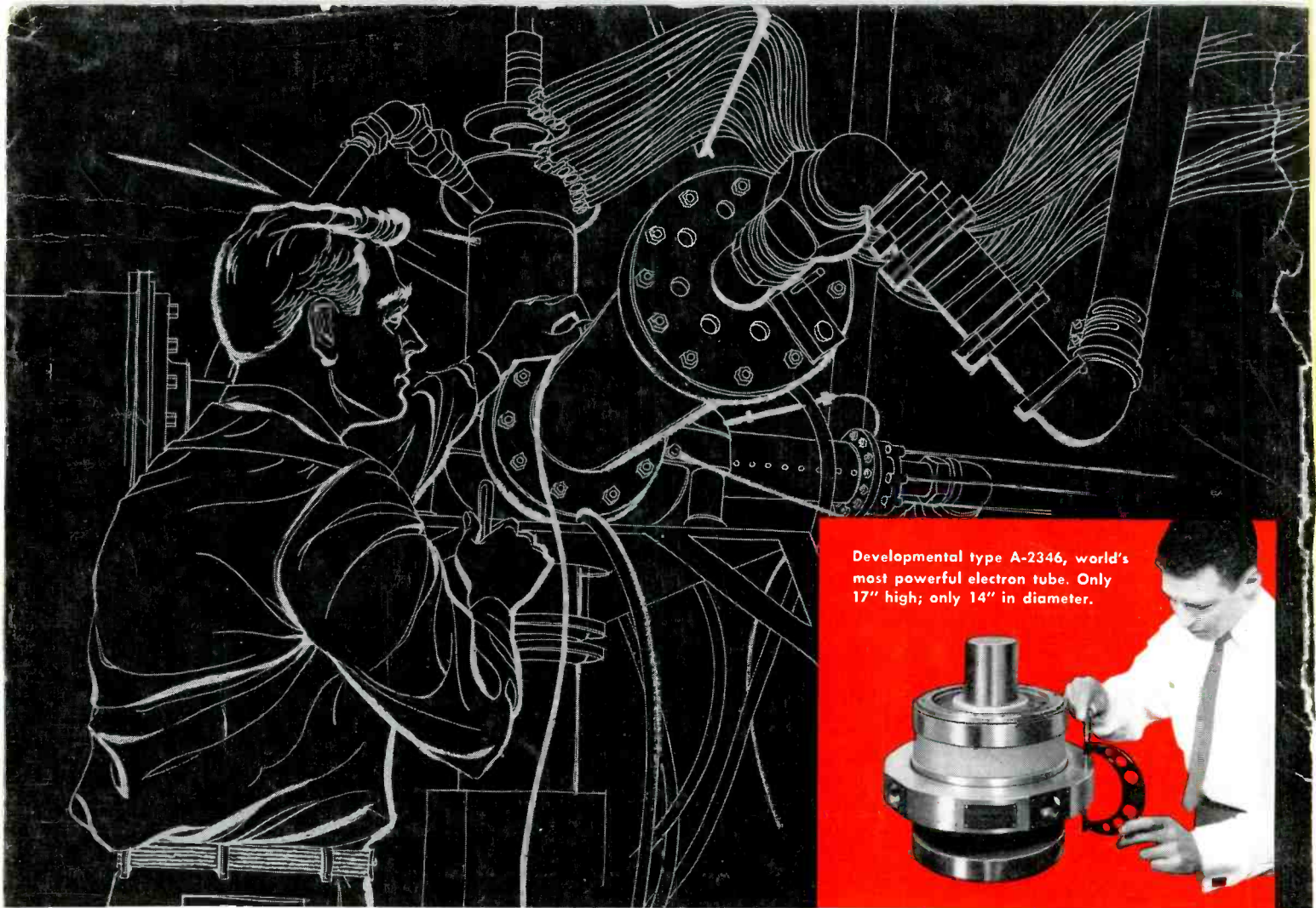
Adjusting an A-2346 Super-Power Tube in an rf power amplifier utilizing experimental cavities.
