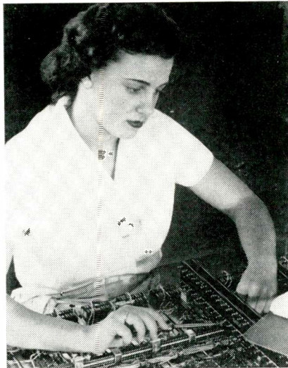
To meet rigid torque tests IBM gold plates brass resistor-board lugs. Plating prevents embrittlement, while protecting against corrosion. Here operator completes assembly of board provided by Taylor Fibre Co. into SAGE computer unit.
