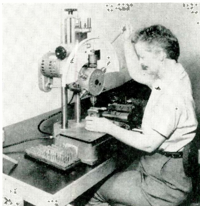
Problem of machining precision holes of different diameters in electronic parts is simplified by this 6-spindle turret drill by Burgmaster Corp., Gardena, Calif.
