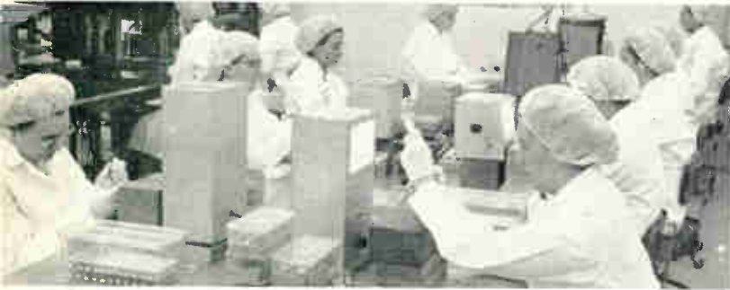
Final tube assembly in near-sterile "clean rooms" assures exceptional tube reliability. These rooms are pressurized with filtered, conditioned air to prevent the tiniest dust particles from entering. Even shoes are automatically vacuum cleaned as personnel enter the room through double-door air locks.
