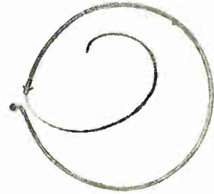
FUEL CELL CABLE: Safely conducts electricity to fuel control valves, pumps, switches and gaging devices immersed within fuel cells. Features: unbroken stainless steel bellows type conduit, double layer protection between current carrying conductors, stainless steel integral connector shells.
