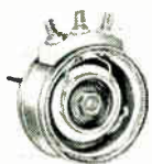
SERIES C-078. 7/8" miniature, height only 5/8", weight 1/2 oz. Multiple finger brush. Single or multiple gangs... completely enclosed. Cored terminals can't loosen. Board integrally molded in housing.
