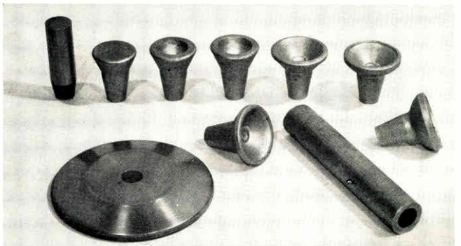
Deep drawn cup from 0.170 in. rolled plate.
