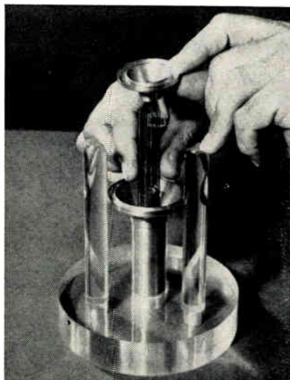
Here the cathode sleeve & flange have been loaded; now, heater & base wafer added.
