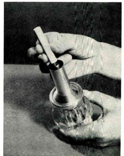
Assembling coated cathode cup over cathode sleeve after assembled mount brazing.
