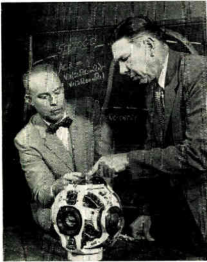
Dr. Carl A. Frishe, president of Sperry Gyroscope and Nathan P. White, engineering chief examine stable platform which will guide nation's first "man in space."
