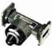
CALIBRATED - SHIELDED ATTENUATORS 611 — 8.2 to 12.4 Kmc/Sec 711 — 12.4 to 18.0 Kmc/Sec .3 to 35 db 1.15 Max VSWR
