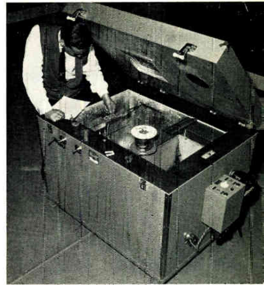
Fig. 10: Test chamber controls temperatures from -73° C to 177° C. It is being set-up for -65° C wire bend tests.
