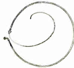
FUEL CELL CABLE: Safely conducts electricity to fuel control valves, pumps, switches and gaging devices immersed within fuel cells. Features: unbroken stainless steel bellows type conduit, double layer protection between current carrying conductors, stainless steel integral connector shells.
