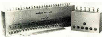
Sealed unit has metal-to-glass terminals
