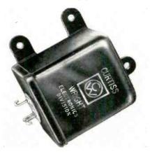
to shock and vibration. Preset time delays between 20 and 180 sec. are available. The relay is voltage compensated from 22 to 32 vdc with a nominal 28 v. rating. Temperature compensation is from  $-65^{\circ}$ C to  $+125^{\circ}$ C. Operating power is less than 3 w. after the timing interval and 10 w during timing. Various contact arrangements are available. Curtiss-Wright Corp., Wood-Ridge, N. J.
