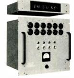
MODEL 202 for Tape Searching operates during data reduction periods. This instrument automatically locates and selects for controlled playback the tape data included between a "sequence start time" and a "sequence end time" specified by panel dial settings. Model 202 may be modified to search for timing formats other than those originated by Model 201.
