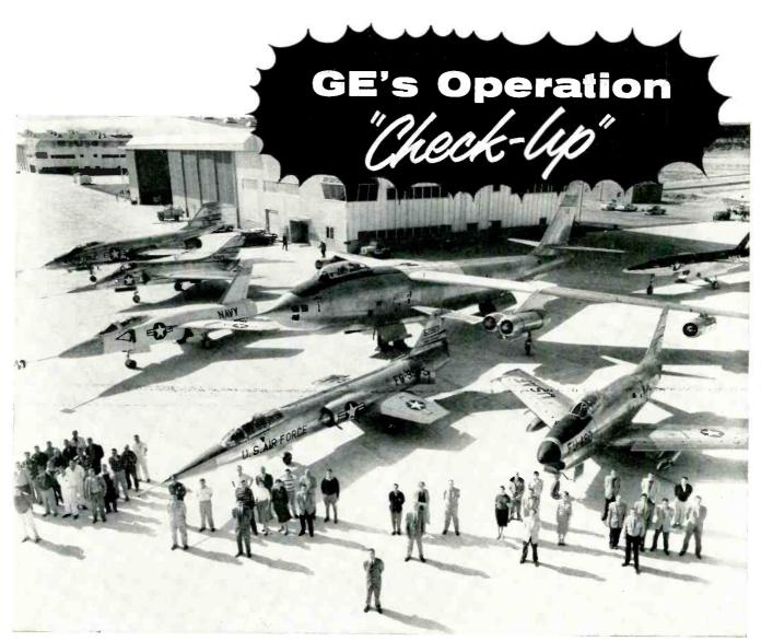
New General Electric Flight-Test hangar at Edwards AFB houses technical and engineering services for aircraft maintenance, instrumentation, data reduction, operations control, quality control, advanced design, etc. Planes shown include the Vought Regulus II Missile, North American F-86, Boeing B-47, Lockheed F-104, Grumman F11F-1F, Douglas XF4D, and the McDonnell F-101.
