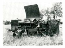
Special design MPQ-4A Mortar Locator Radar developed for the Signal Corps by C.E. detects mortar shell in flight and computes the location of the enemy's mortor installation.
