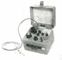
channel requirements. With a builtin thermometer, the crystal controlled instrument covers any r-f channel within the 25 MC to 470 MC communications spectrum, accurate to  $\pm 0.00025$  percent. It is also a precision instrument for i-f channels in the 100 KC to 100 MC range. Allen B. Dumont Laboratories, Inc., 750 Bloomfield Ave., Clifton, N. J.
