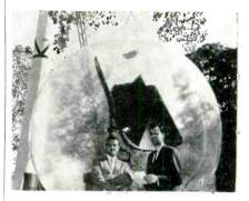
Hughes' E. W. Templin and Dr. N. A. Begovich stand in front of novel antenna of their new "Frescanar" radar which simultaneously computes distance, bearing, height.
