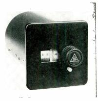
is supplied in the standard resistance value of 10,000 ohms and in other resistance values on special order. Full scale resistance accuracy is  $\pm 0.05\%$ , linearity  $\pm 0.01\%$ , resolution 0.002%. Power rating is 5w and the operating frequency range is dc to 10 KC. Rinco Inc., 7962 S.E. Powell Blvd., Portland, Oregon.
