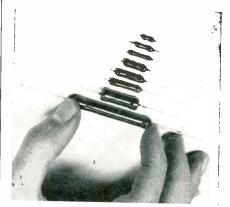
has eight sizes, with a selection of five wattage ratings: 1/8, 1/4, 1/2, 1 and 2 watts. Resistance range is from 1 ohm to 50 megohms, depending on size and type. Standard tolerance is 1%. Typical derating is 100% power to 70°C. derating to 0% at 150°C. Dielectric strength is 1000 vac on the V-block test. All resistors have axial leads. Dale Products, Inc., Columbus. Nebraska.
