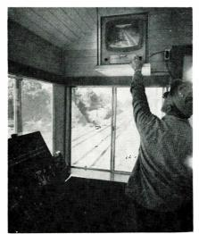
Crossing tender for the D & H Railroad, Cohoes, N. Y., adjusts G.E. closed-circuit TV monitor which gives him a picture of switching engines approaching the main line.
