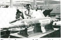
The Air Forces new 7.62 mm. Vulcan is shown in its mockup stage at GE's Missile & Space Vehicle Dept., Burlington, Vt. The new Gatling-type weapon will fire 3,000 rds/min.
