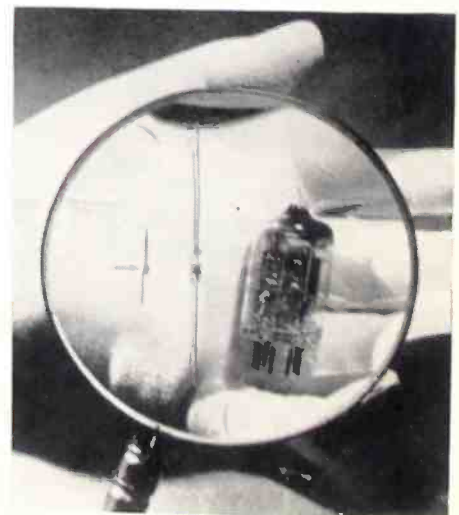
No larger than a household pin is this new hermetically sealed diode developed by Pacific Semiconductors Inc. and shown alongside conventional diode and 6AL5.
