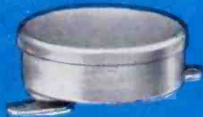
TYPE MX Hermetically Sealed — Electrically independent bimetal disc. Rated at 2 amps at 115 VAC and 28 VDC, based on 250,000 operations.
