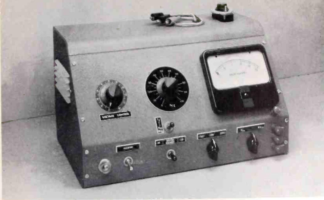
Fig. 1: This test equipment is designed to give the dc current transfer ratio.
