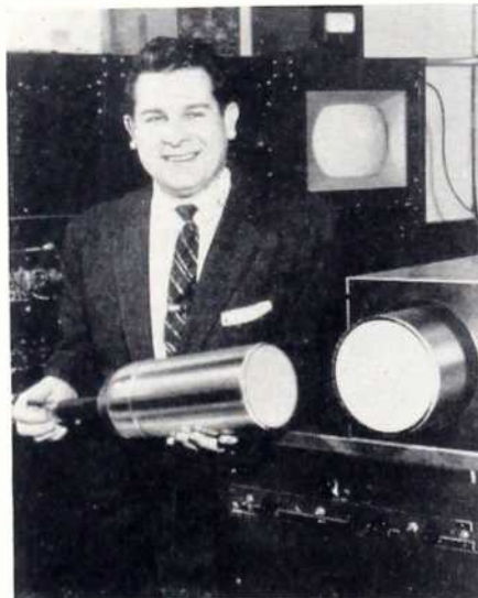
CBS-Hytron's N. F. Fyler displays new ultra-high resolution CRT that transmits photo information of microscopic detail.
