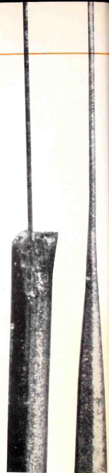
Fig. 2: The etched, tapered transition between leads and strain gage filament is stronger and more stable than welded joints.
