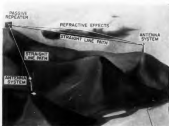
Fig. 3: Transmission path is the path joining the centers of the final radiators. Path length is the total of the two path lengths
