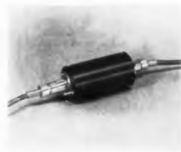
Fig. 3. Booster assembles into a can 2 inches in diameter by 3 1/8 inches long. Cannon XL3 connectors are used. The projecting screw serves as switch by contacting battery.
