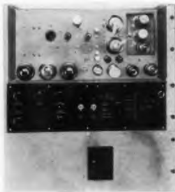
Fig. 4: Metering and control circuits are contained along with the video stages
