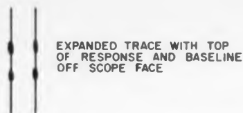
Fig. 6 (above): "Blown up" trace minimizes error in leveling dots.
