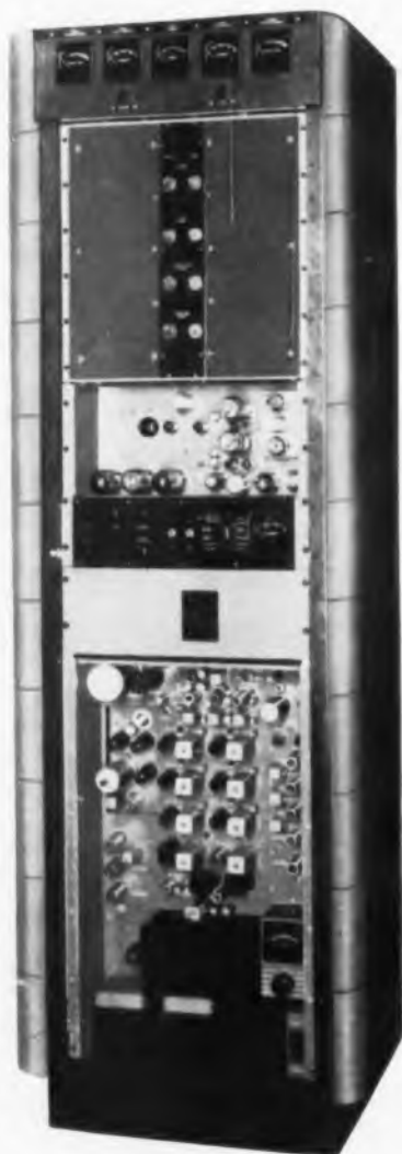
Fig. 1: A compact VHF transmitter that may be used for a driver unit.
