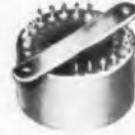
Multi-control magnetic amplifier for airborne servo.
