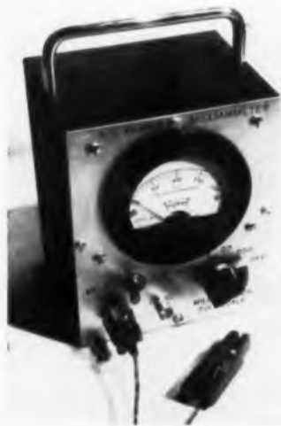
Fig. 4: Photograph of ac microammeter with clamp-type probe developed at NBS. Probe is in foreground.
