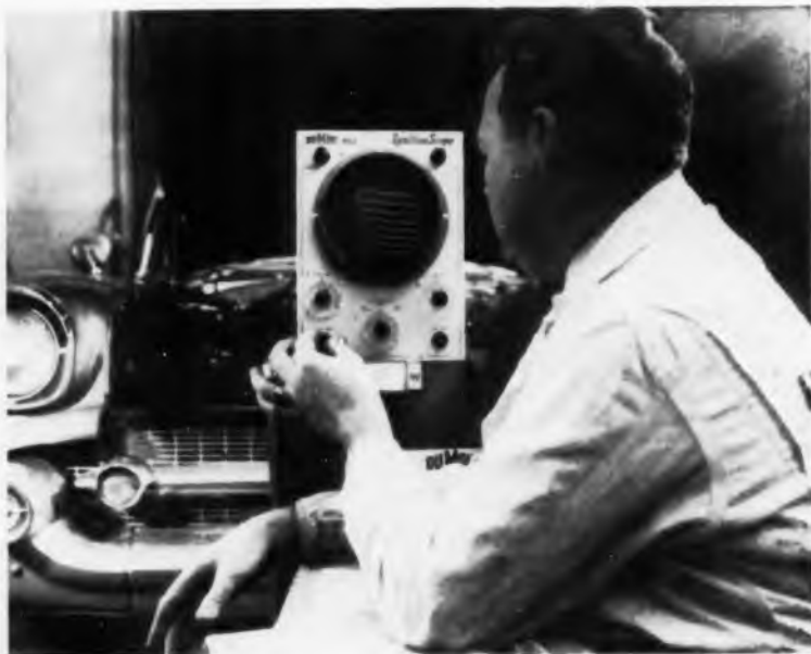
Each separate trace in the IgnitionScope shows ignition in a separate cylinder. From comparing these traces, the auto mechanic can diagnose a wide variety of motor ills.
