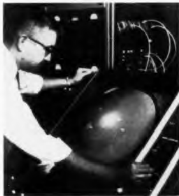
New tube identifies aircraft by flashing symbols alongside "blip" shown on scope
