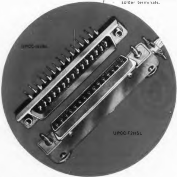
Series UPCC-SLK* (Knob Screw Lock). Female chassis connector wire solder terminals. Knob on male card connector dip solder terminals.
