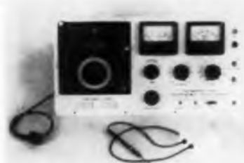
Fig. 17: Ford Instrument Co.'s Ophthalmic-Electrotome, an electrosurgical device, performs the extremely delicate task of reattaching eye retinas.
