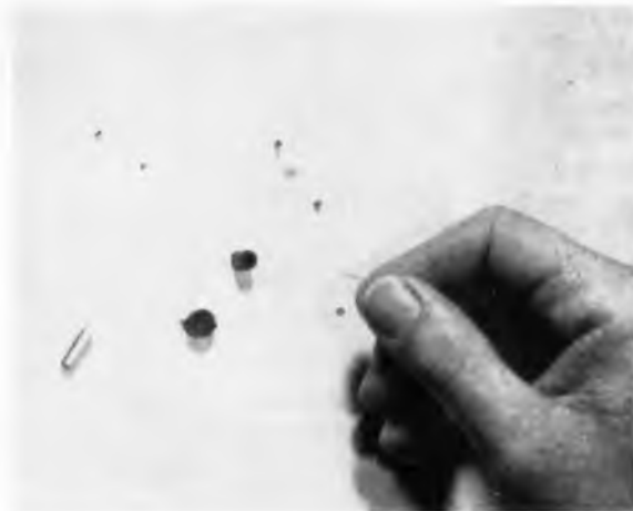
Fig. 1: These coils, in various sizes and shapes, were threaded by SRI's versatile "Pinhole" coil winder.
